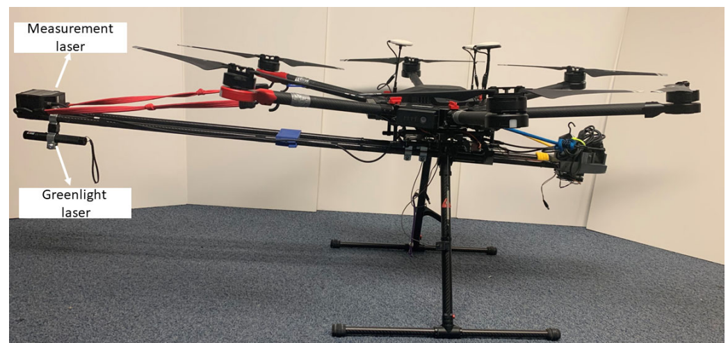
Figure 1. Portable greenlight laser added in the UAS, next to the displacement measuring laser.
