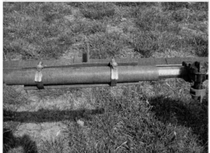
Figure 3: Wet boom with heater hose set-up and stainless steel hose clamps to hold boom in place.
