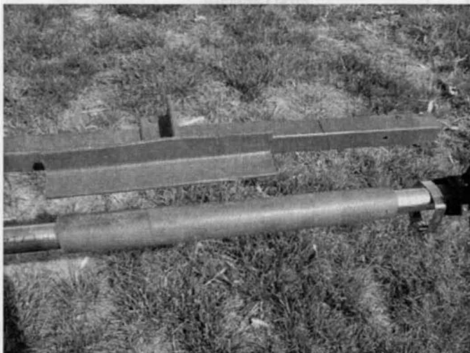
Figure 3: Wet boom with heater hose set-up and stainless steel hose clamps to hold boom in place.
