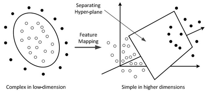
Fig. 5. Feature mapping by using the kernel function.
