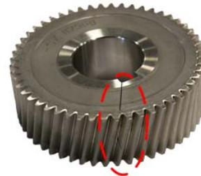
Fig. 8. The test gear with a crack.
