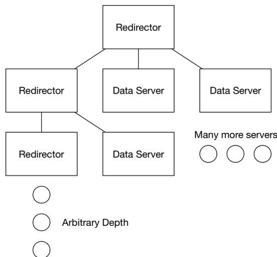
Figure 1: Diagram of XRootD's organization (Modeled after [4])
