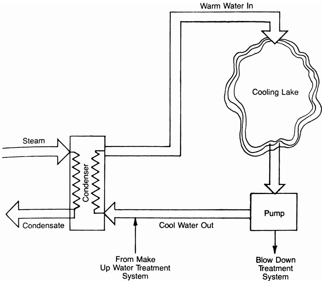
Figure 2. Closed Cycle Cooling Lake.
