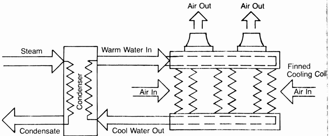
Figure 5. Dry Cooling Tower Natural or Mechanical Draft.
