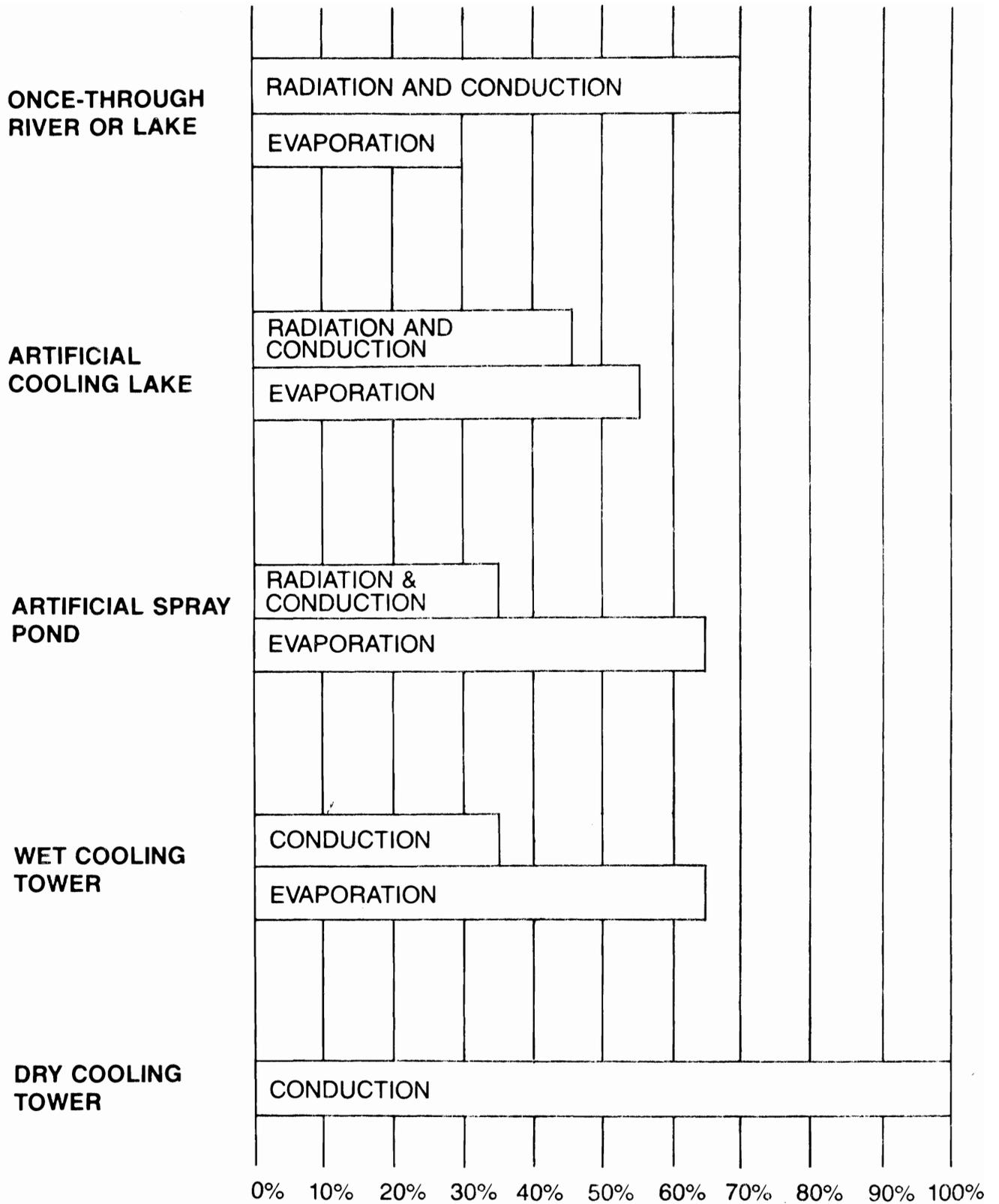
Figure 6. Heat Transfer Mechanisms with Alternative Cooling Systems.
