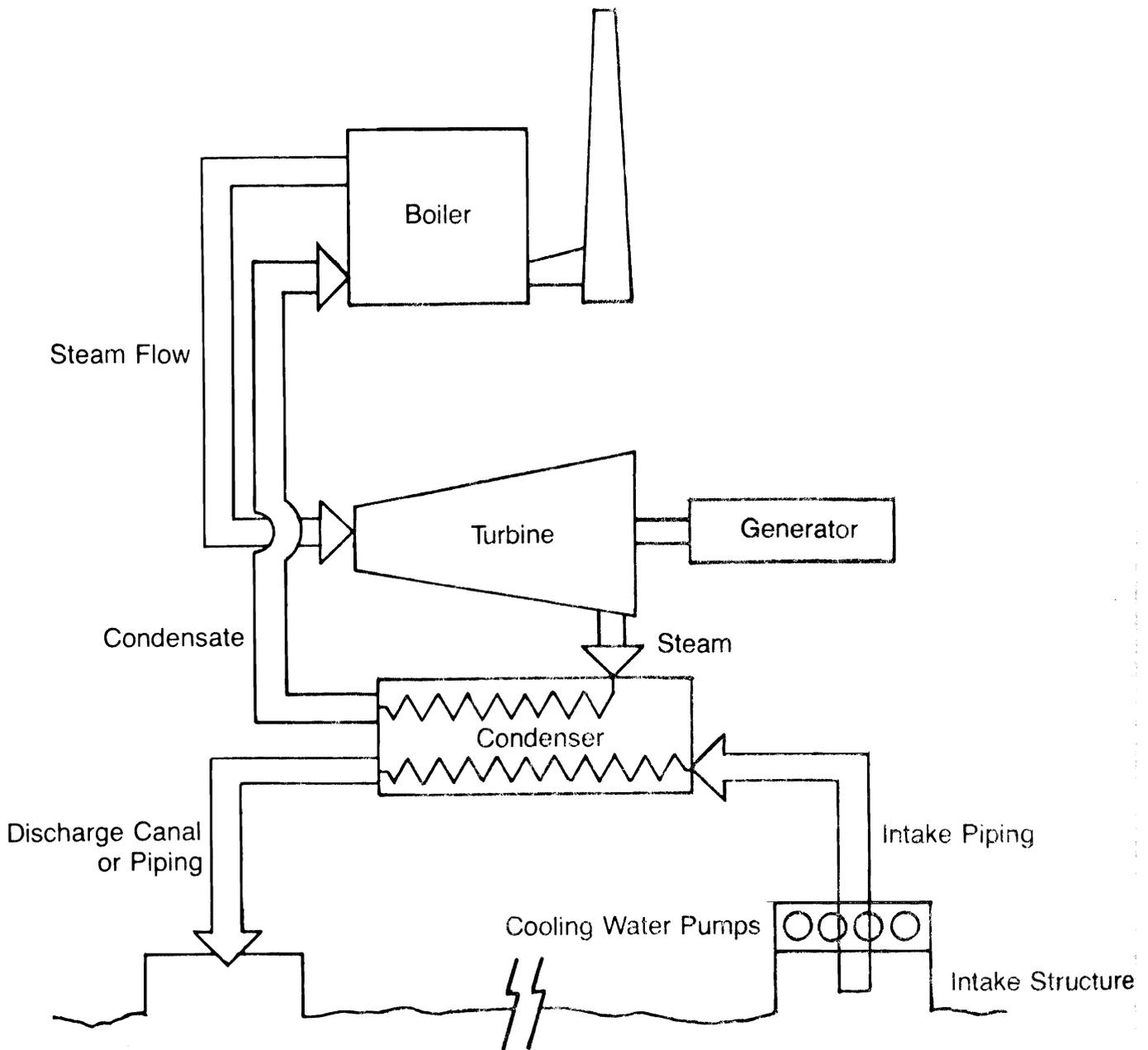
Figure 1. Once-Through Circulating Water System.
