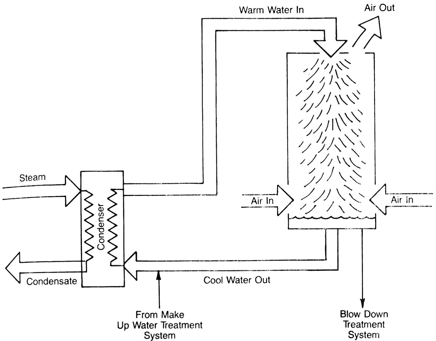
Figure 3. Wet Cooling Tower Natural or Mechanical Draft.
