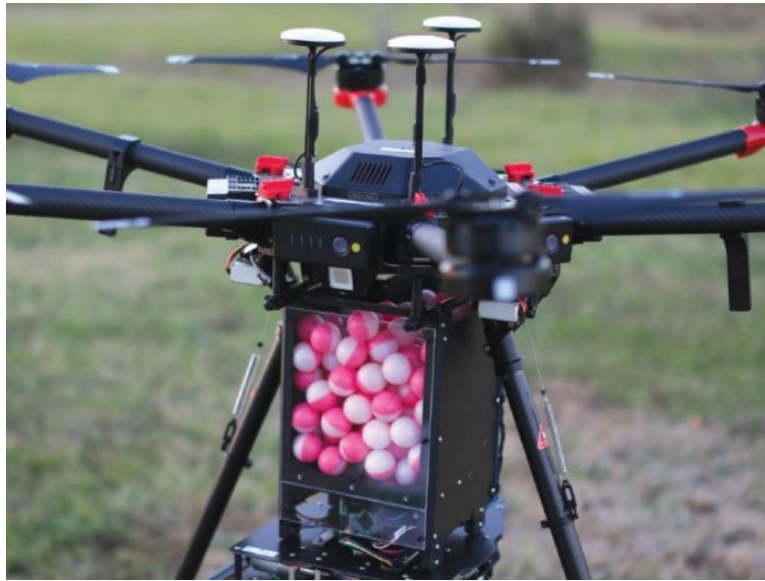
Figure 5: “IGNIS” a software created by drone amplified that is used to chemically set prescribed burns that help prevent wildfire spread (Carrick Detweiler).
