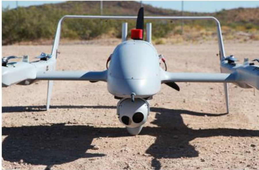
Figure 3: Using mapping software and an advanced imagery system, the UAVs supplied by Bridger Aerospace is able to map areas with multiple layers day or night and gather fast outlines of fires (Weston Irr).
