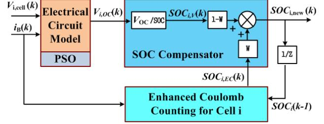
Fig. 2. The proposed closed-loop weighting SOC estimation algorithm.
