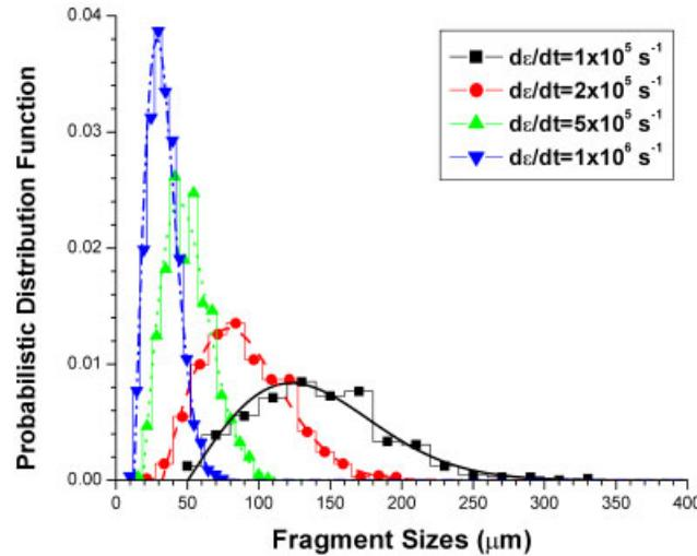
Figure 6. PDF of fragment size for a ceramic ring under different strain rates [41].
