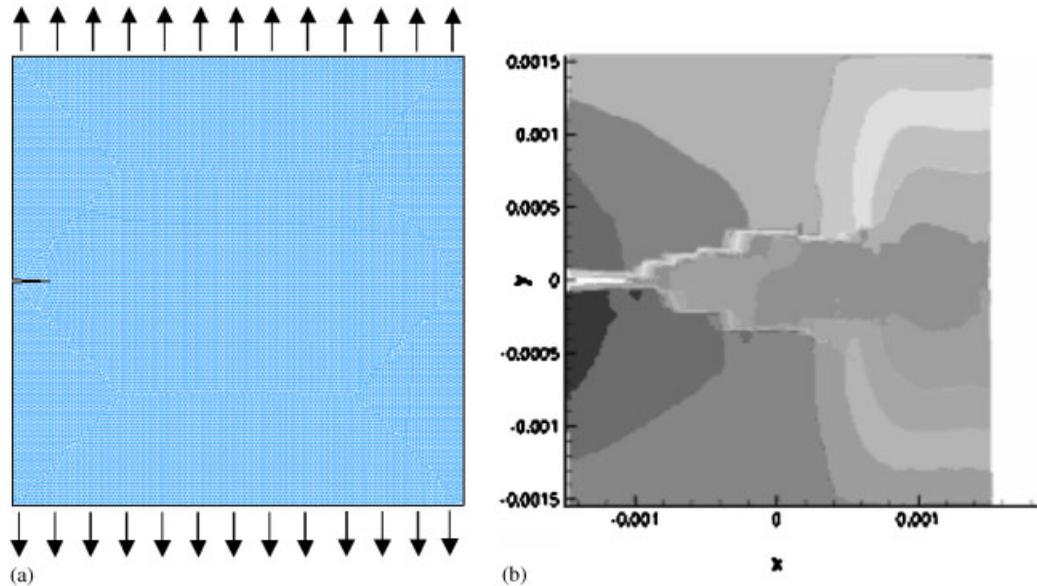
Figure 2. (a) Finite-element mesh of a PMMA plate under mode I opening (the mesh contains 36 096 T6 elements); and (b) simulation results showing crack branching, which were obtained for  $W_0/G_c = 13.5$  (vertical displacement contours are shown; displacements on top and bottom boundaries are  $\pm 43 \mu\text{m}$ ).
