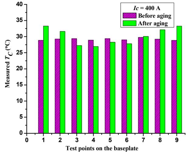
Fig. 8.  $T_C$  distribution among nine dies before and after the aging test.
