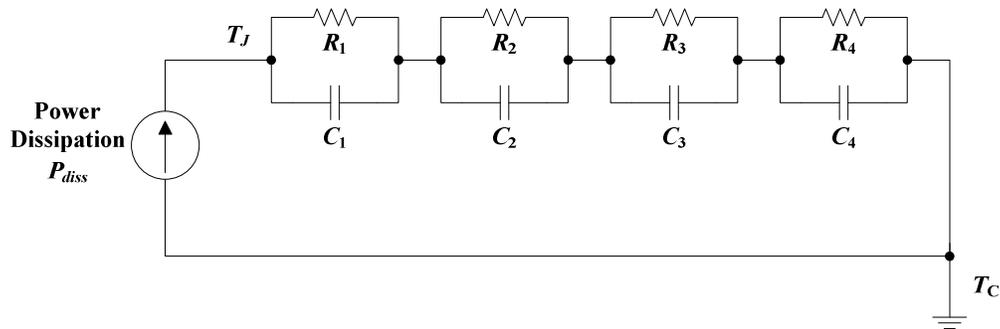
Fig. 2. Schematic of a Foster equivalent RC thermal network for IGBTs.
