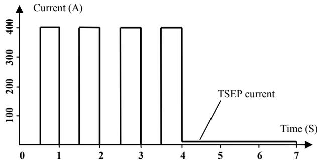
Fig. 6. Pulsed-current waveform used in the tests.
