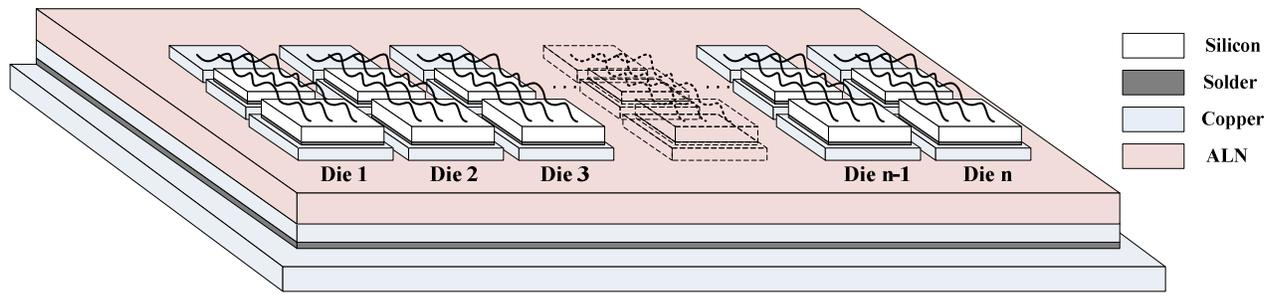
Fig. 1. The DBC structure of a multidie IGBT module.
