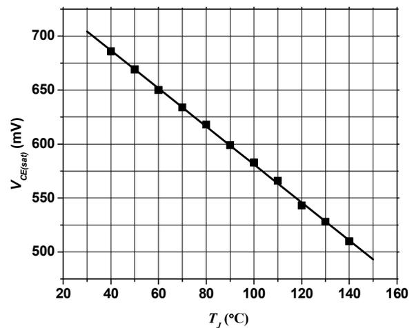
Fig. 5. Measured  $V_{CE(sat)}$  as a function of  $T_J$  for the test IGBT.
