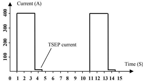
Fig. 7. IGBT current waveform during the aging test.
