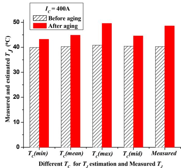
Fig. 9. Comparison of measured  $T_J$  and  $T_J$  estimated by using different  $T_C$  before and after the aging test.
