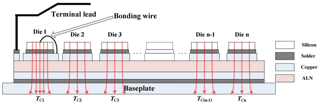
Fig. 3. Heat flows through a multidie IGBT module.
