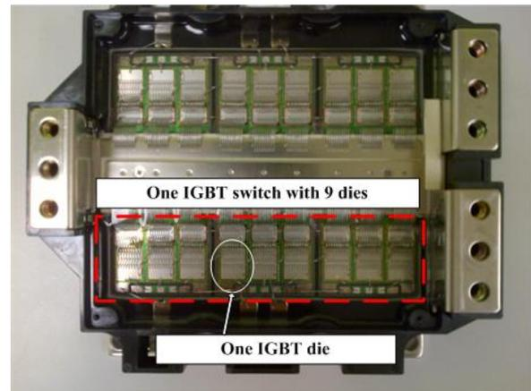
Fig. 4. Internal structure of a test multichip IGBT module.
