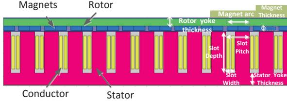
Fig. 1. 2D-FEA Model of a 24 slots/22 poles double layer winding AFPM
