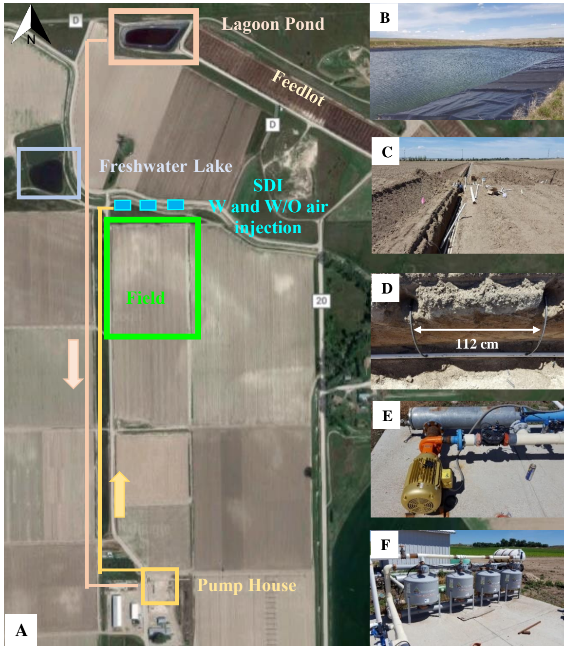
Figure 2: (A) Irrigation layout of the field, (B) lagoon pond, (C) drip line layout in the field, (D) dripline space, (E) water pump used for irrigation, and (F) sand filters for the filtration.
