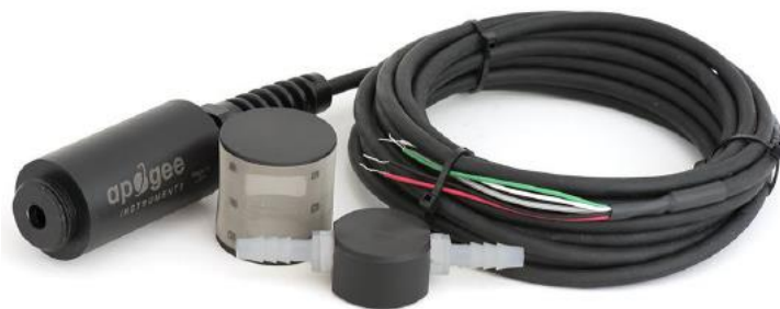
Figure 10: Oxygen sensor ( https://www.apogeeinstruments.com/oxygensensor/ ) used to measure soil oxygen content.
