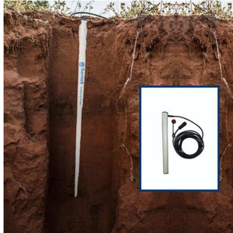
Figure 9: Soil moisture probe ( https://sentektechnologies.com/product-range/soil-data-probes/drill-and-drop/ ) used to measure soil moisture, salinity, and soil temperature.
