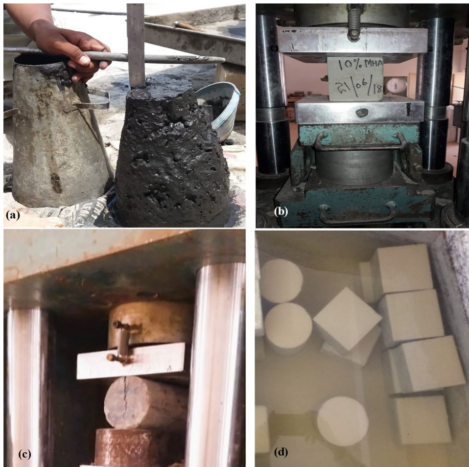
Figure 3. Investigational arrangement (a) Slump test, (b) Compressive strength test, (c) Splitting tensile strength, (d) Water curing tank.
