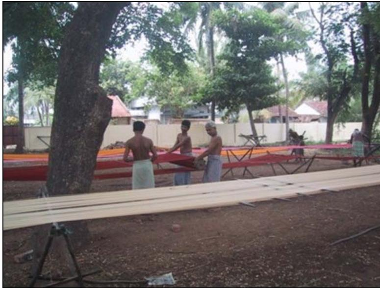
*Figure 4. Rolling up sized warp. Photo: Uzramma.*
