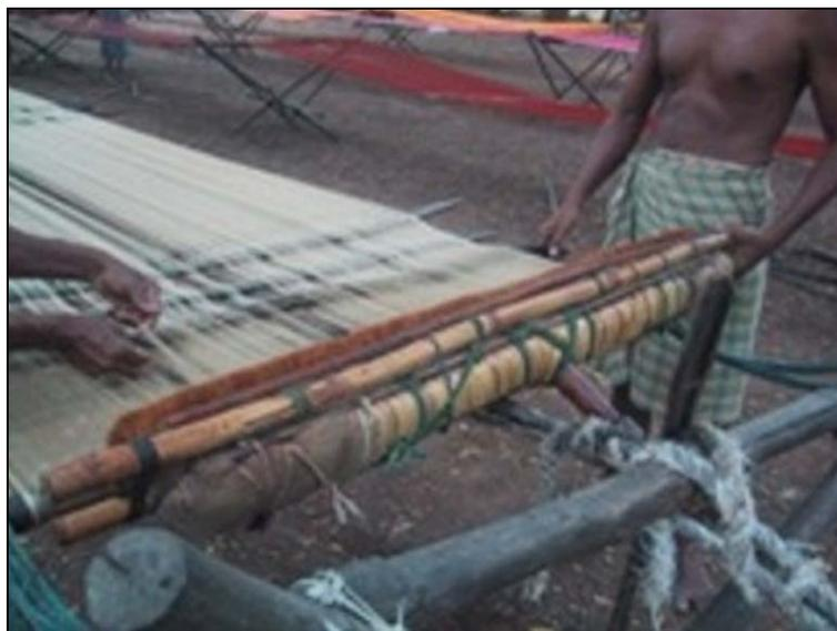
*Figure 3. Mending warp threads. Photo: Uzramma.*
