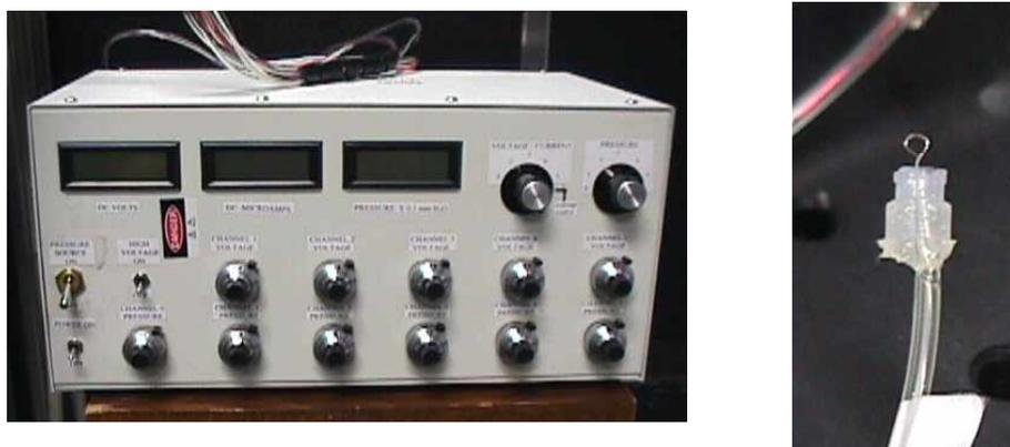
Fig. 5. Custom voltage/pressure controller. Left, front panel showing six channels. Right, PDMS-molded channel terminus showing platinum electrode.
