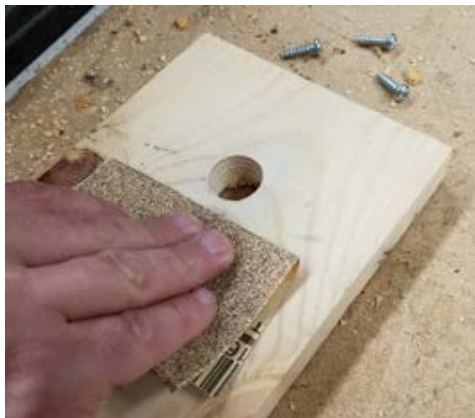
Before putting your birdhouse together, roughen the inside portion of the hole just below the entrance so young birds can climb out of the house easily. You can use coarse sandpaper, cut grooves or punch dents in the wood with a screwdriver.
