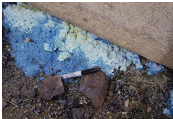
FIGURE 1. Alpersite at the Big Mike mine, Nevada, occurs as a bright blue efflorescence associated with pickeringite [\text{MgAl}_2(\text{SO}_4)_4 \cdot 22\text{H}_2\text{O}] , alunogen [\text{Al}_2(\text{SO}_4)_3 \cdot 17\text{H}_2\text{O}] , and epsomite \text{MgSO}_4 \cdot 7\text{H}_2\text{O} . Pickeringite and alunogen (white and yellow) occur on top of a mat of alpersite (blue) adjacent to a concrete wall. The black end of the pen is 5 cm long.
