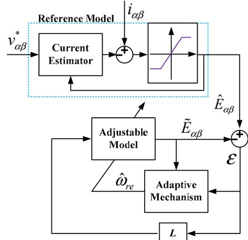
Fig. 2. Schematic of the conventional MRAS-based speed estimator.
