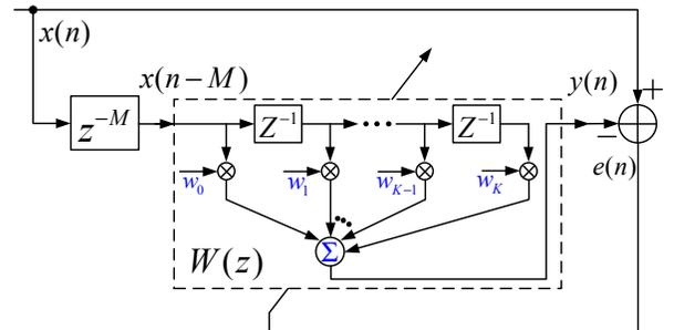
Fig. 4. Block diagram of an adaptive line enhancer.
