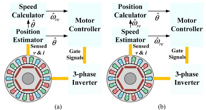
Fig. 1. Illustration of the reduced-order observer-based rotor position/speed estimators based on (a) position and (b) speed estimation.
