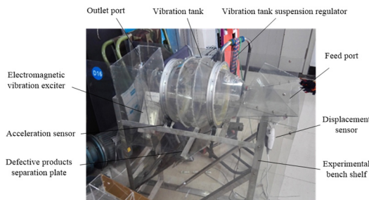
Fig. 1. Nondestructive testing experimental bench
