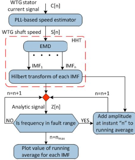
Fig. 1. Flowchart of the HHT-based fault detection algorithm.
