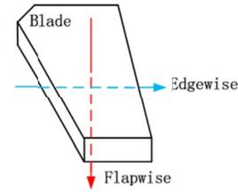
Fig. 6. Depiction of blade bending flapwise or edgewise.
