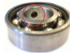
Fig. 9. Testing bearing with an inner-race fault.
