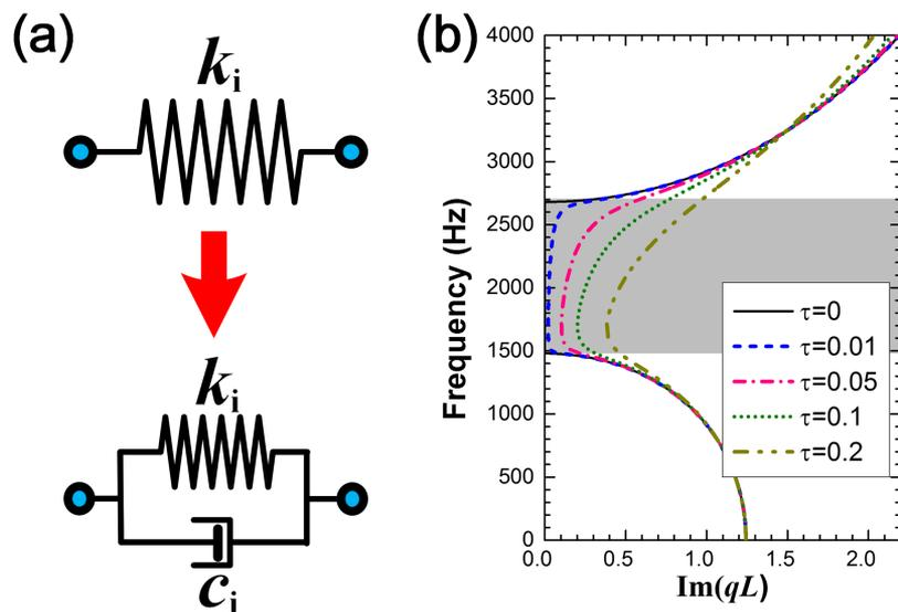
FIG. 2. (a) The effect of dissipation is investigated by changing each linear elastic spring by a Kelvin-Voigt viscoelastic solid analog; (b) imaginary part of the dimensionless wavenumber of the dissipative metamaterial. The grey region corresponds to the passband of the non-dissipative case.
