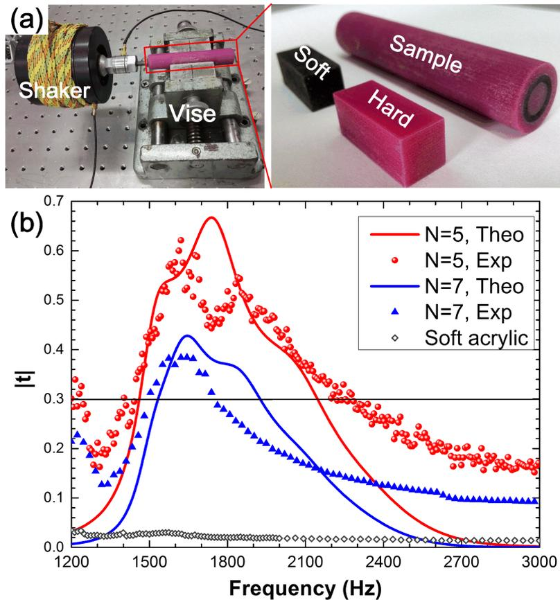
FIG. 4. (a) Photographic images of the vibration exciter and the specimen; (b) experimental and theoretical transmittances for different samples.
