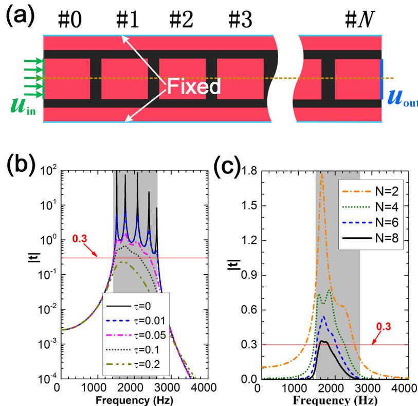
FIG. 3. (a) Schematic of a finite elastic metamaterial with  $N$  periods; (b) transmittance of a 5-period elastic metamaterial with different damping coefficients; (c) transmittance of elastic metamaterials with different number periodic units, the damping coefficient is set as  $\tau = 0.1$ . The grey regions in (b) and (c) correspond to the passband of the non-dissipative elastic case.
