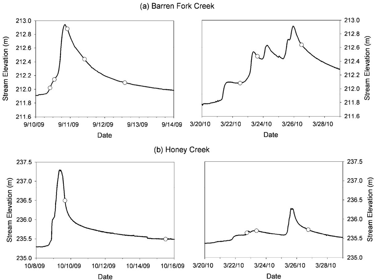
Figure 2. Hydrographs for the Barren Fork Creek (a) and Honey Creek (b) field sites. Circles designate dates of P sampling from the observation wells and creeks.
