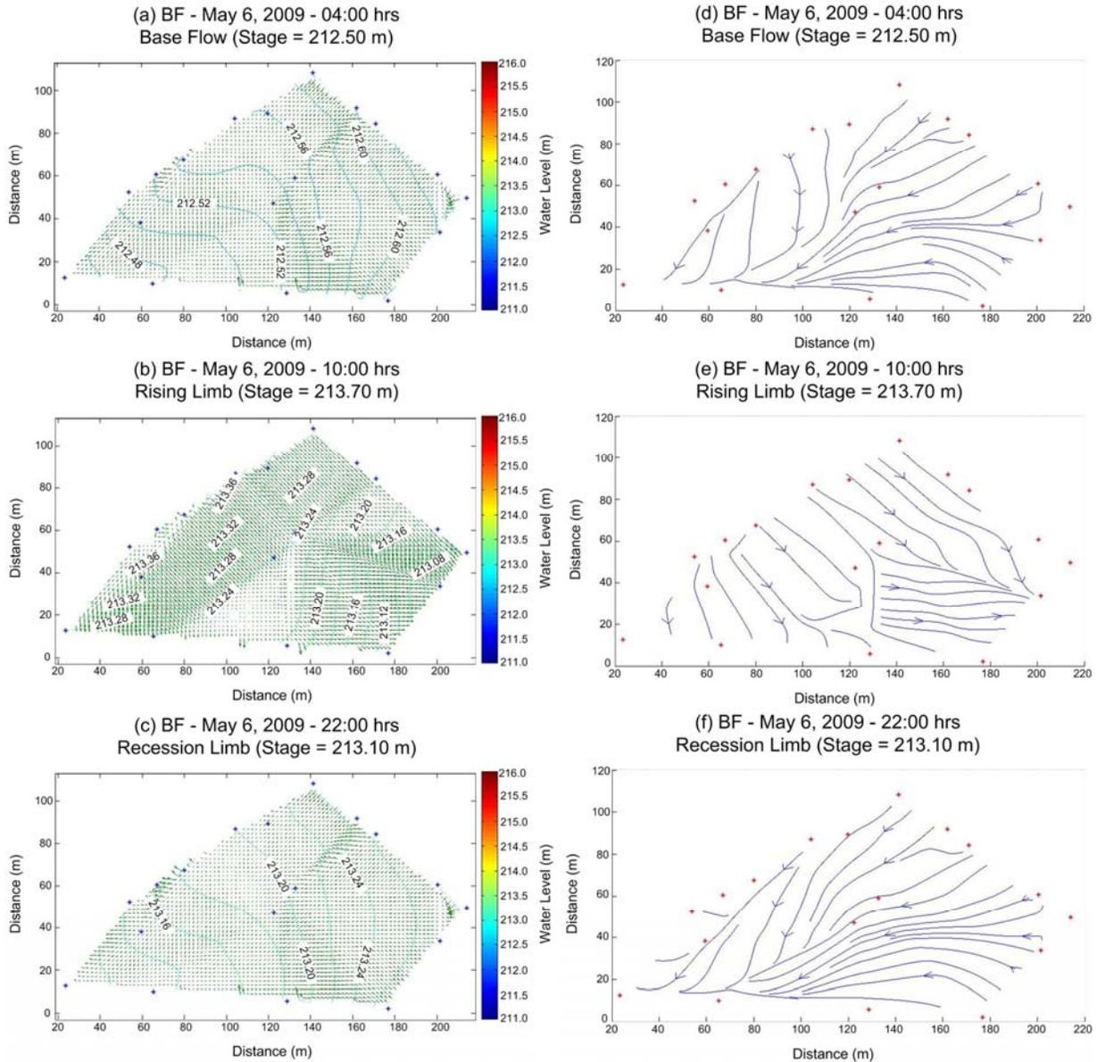
Figure 3: Water table elevation contour plots (a-c) and streamlines (d-f) for the Barren Fork (BF) Creek site during baseflow (a and d), the rising limb (b and e), and the recession limb (c and f) of a streamflow hydrograph. For scale, the May 6, 2009, event had a peak flow of  $250 \text{ m}^3 \text{ s}^{-1}$ , a 1.3-yr recurrence-interval event. Arrow vectors in the background (a-c) indicate the magnitude and direction of the water table gradient.
