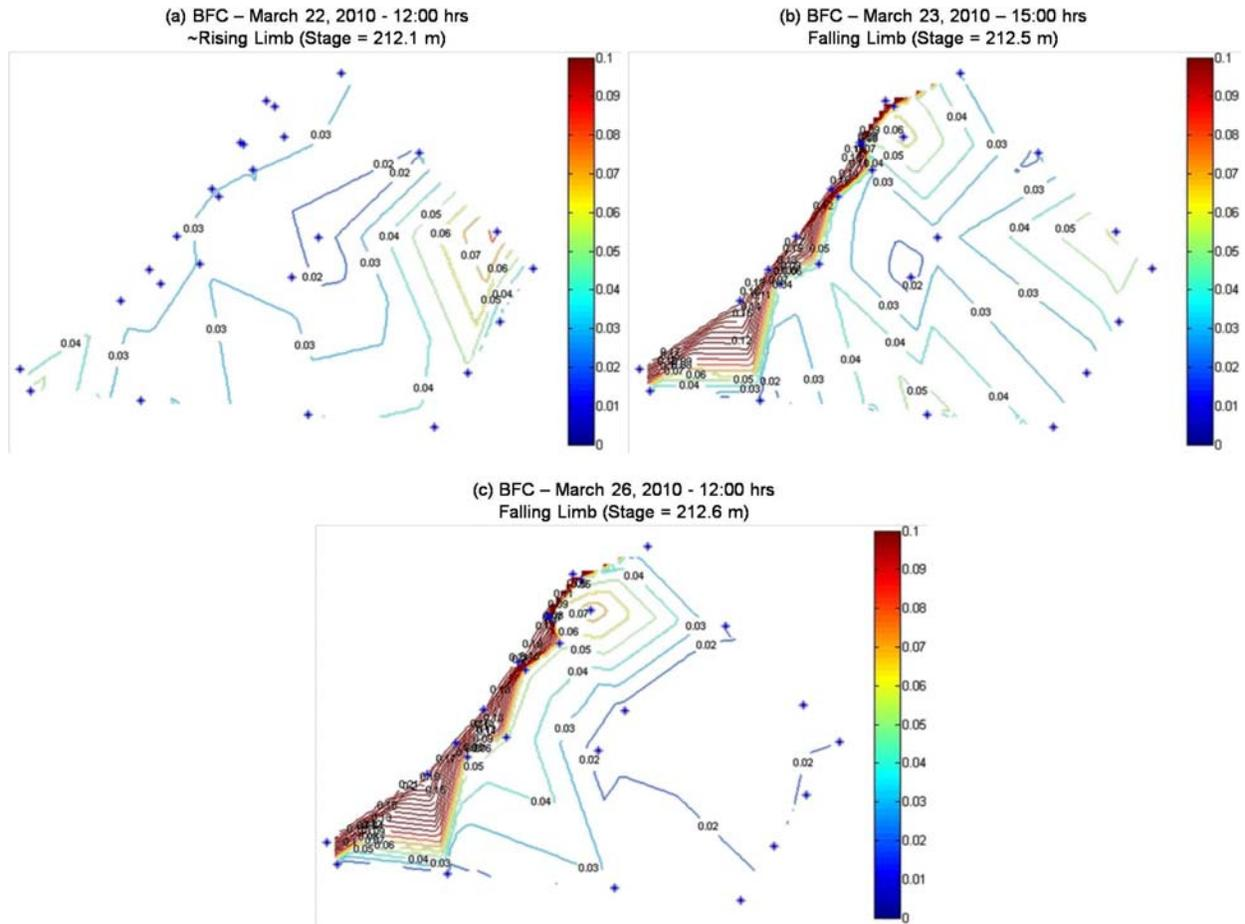
Figure 6. Total P concentration (mg/L as P) contour plots for the Barren Fork Creek (BFC) for the March 23 and March 25, 2010, flow events. The maximum flow for the March 23, 2010, event (a and b) was  $48 \text{ m}^3 \text{ s}^{-1}$ , a 1.05 year recurrence interval event. The maximum flow for the March 25, 2010, event (c) was  $85 \text{ m}^3 \text{ s}^{-1}$ , a 1.1-yr recurrence interval event.
