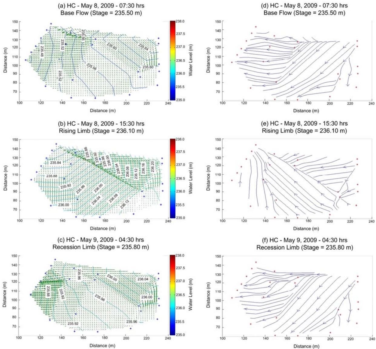
Figure 4: Water table elevation contour plots (a-c) and streamlines (d-f) for the Honey Creek (HC) site during baseflow (a and d), the rising limb (b and e), and the recession limb (c and f) of a streamflow hydrograph. For scale, the May 8, 2009, event had a peak flow of  $18 \text{ m}^3 \text{ s}^{-1}$ , a 1.7-yr recurrence interval event. Arrow vectors in the background (a-c) indicate the magnitude and direction of the water table gradient.
