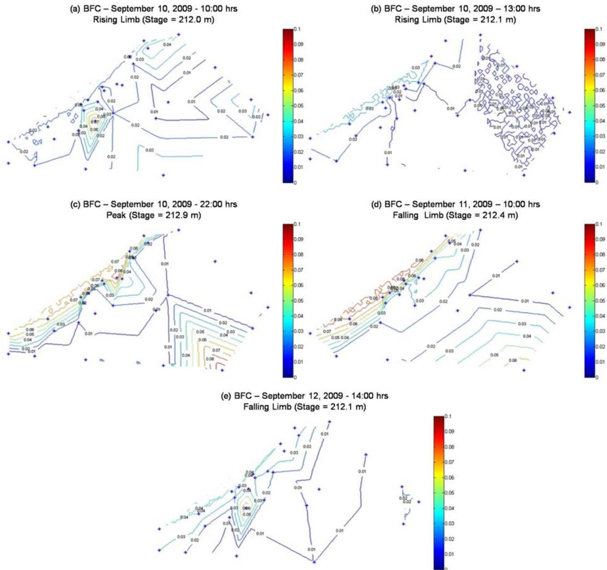
Figure 5. Total P concentration (mg/L as P) contour plots for the Barren Fork Creek (BFC) for the September 10, 2009, high flow event. Maximum flow was  $86 \text{ m}^3 \text{ s}^{-1}$ , a 1.1-yr recurrence interval event.
