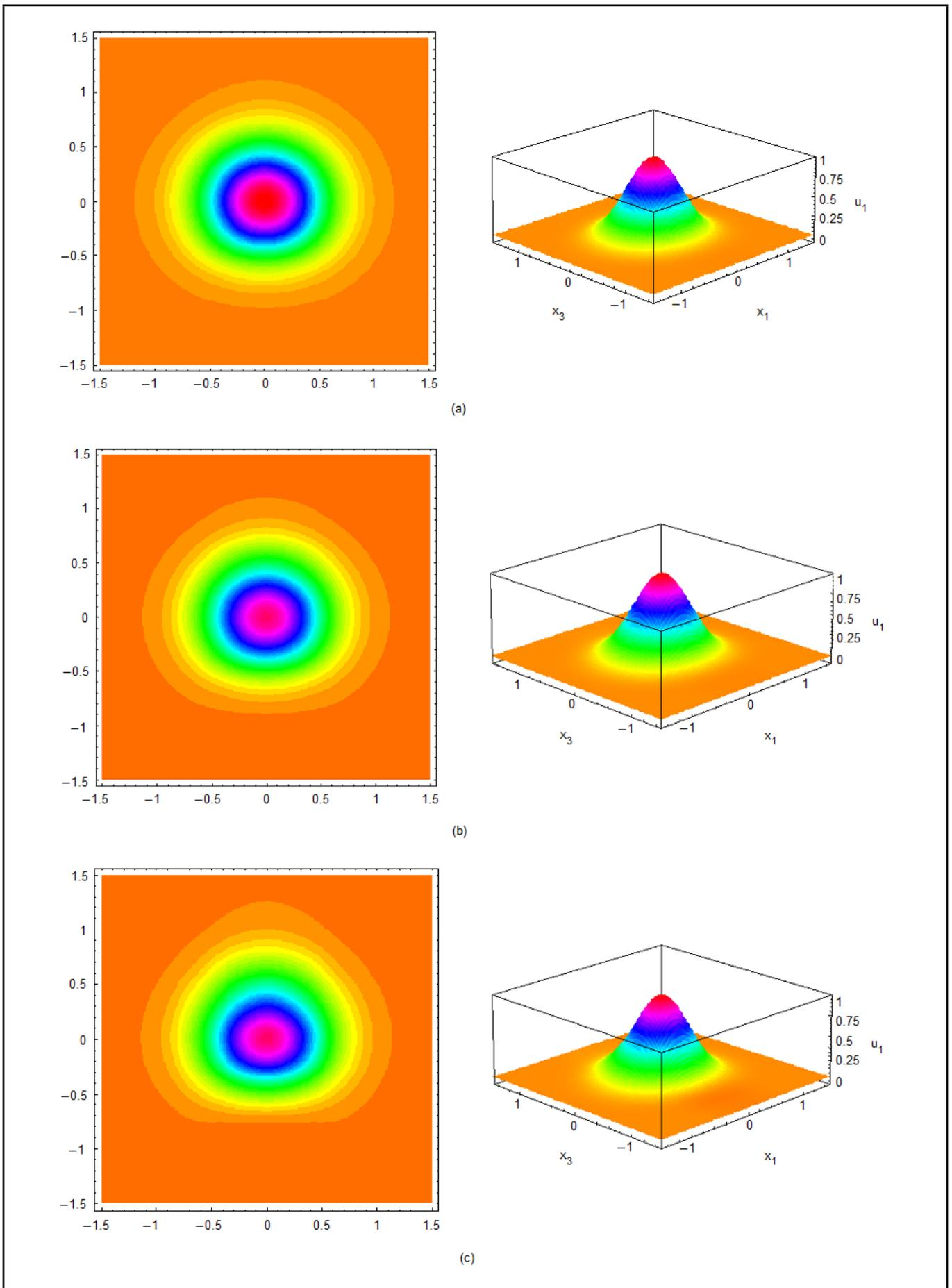
**Figure 4.** Effect of  $d(b = 0)$ . (a)  $d = 0.1a$ ,  $\omega_1 = 1.526053 \times 10^7 1/s$ . (b)  $d = 0.2a$ ,  $\omega_1 = 1.526128 \times 10^7 1/s$ . (c)  $d = 0.5a$ ,  $\omega_1 = 1.526693 \times 10^7 1/s$ .
