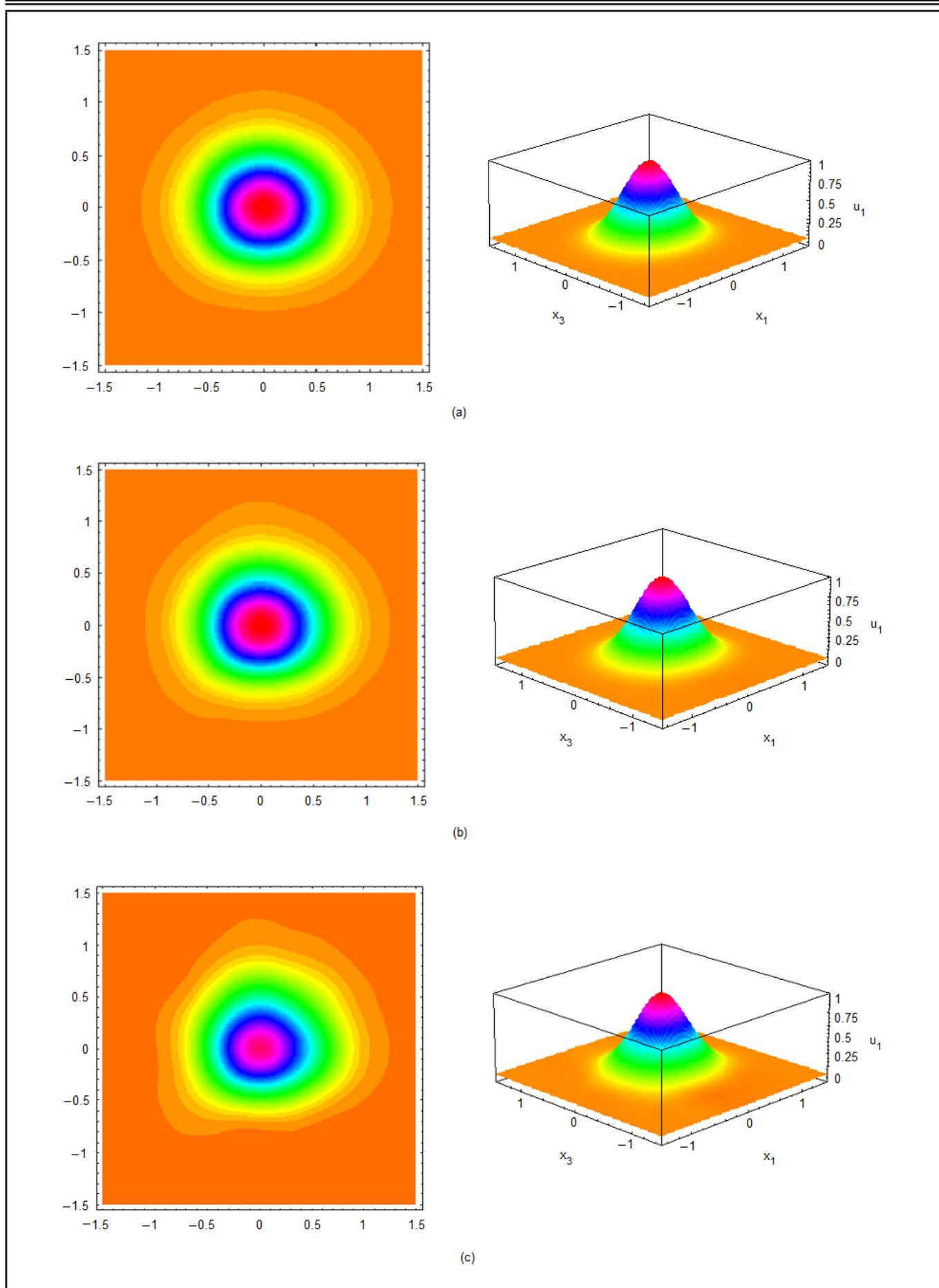
**Figure 6.** Both  $b$  and  $d$  are varying. (a)  $d = b = 0.1a, \omega_1 = 1.526081 \times 10^7 \text{1/s}$ . (b)  $d = b = 0.2a, \omega_1 = 1.526238 \times 10^7 \text{1/s}$ . (c)  $d = b = 0.5a, \omega_1 = 1.527357 \times 10^7 \text{1/s}$ .
