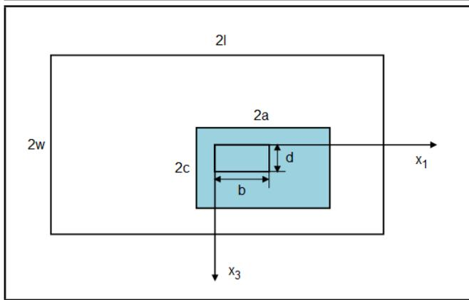
Figure 2. A rectangular resonator with electrode off centre.
