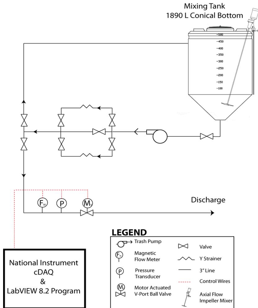
Figure 1. Sediment mixing system schematic with tank gradations in gallons.
