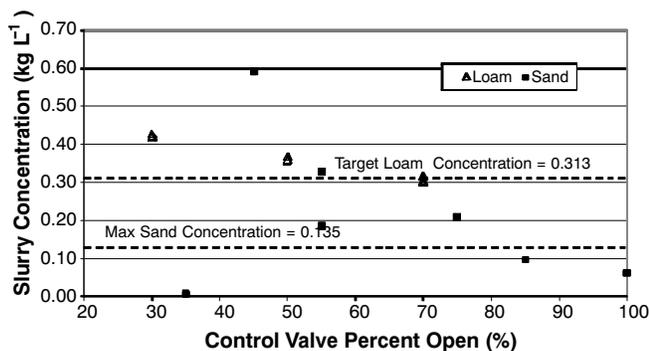
Figure 5. Soil slurry outflow concentration for loam and sand based on one replication.
