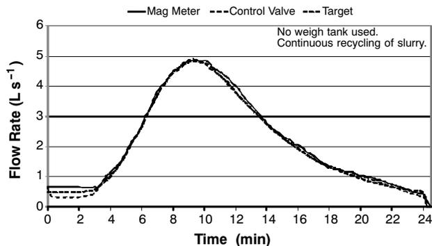
Figure 4. Slurry flow rate for silty clay sedigraph, replicate 3, including target, Magnetic meter reading (measured flow rate), and control valve setting flow rate. Replication 1 and 2 produced similar graphs.
