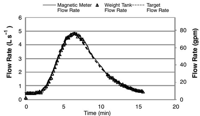
Figure 3. Hydrograph with NSE of 0.998 between magnetic meter measured flow rate and target flow rate.
