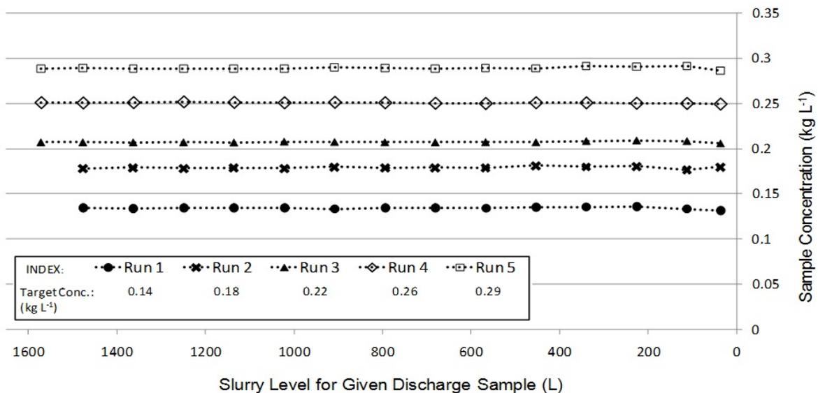
Figure 2. Concentration fluctuation as the mixing tank drains.
