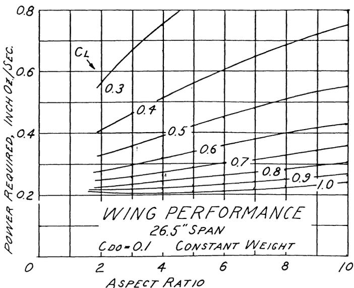
Figure 2. Wing performance 26.5 inch span  $C_{DO} = 0.1$  constant weight.
