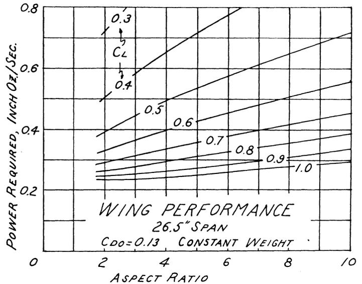
Figure 3. Wing performance 26.5 inch span  $C_{DO} = 0.13$  constant weight.
