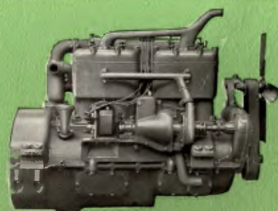
SHOWING MAGNETO SIDE AND ENCLOSED GOVERNOR The governor is entirely enclosed to exclude dust and acts to prevent the engine racing if the load is suddenly thrown off. By the removal of five stud bolts, the outside cover of the governor can be quickly removed.
