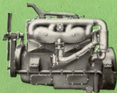
SHOWING CARBURETOR AND MANIFOLD SIDE The Illinois Super-Drive Tractor is equipped with a powerful four-cylinder slow speed, kerosene burning engine. This engine is ample to do all the work it may be called upon to do without strain.
