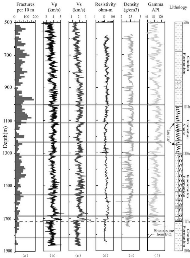
**Figure 4.** (a) Fractures density picked from FMS and FMI in 10 meter intervals. (b) P-wave velocity, (c) S-wave velocity, (d) Resistivity, (e) Density, and (f) Gammy ray and lithology from core descriptions. The zones with localized stress rotations are shown on geophysical logs with thick gray lines. The fault zones identified from the on-site core description (E.-C. Yeh, personal communication, 2006) are shown by gray bars in the lithology column.
