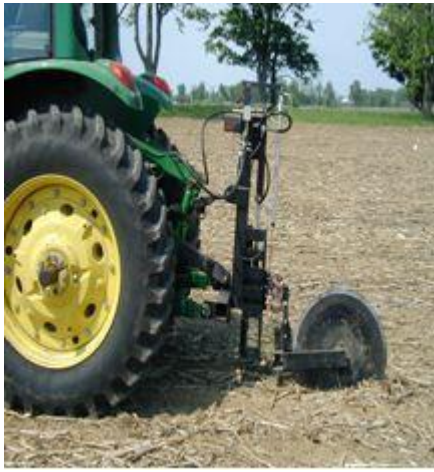
Figure 4. Data collection scheme (left); soil coulterometer operation during field data collection at UKARC (right).
