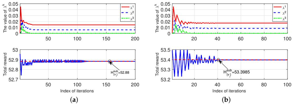
Figure 4. Convergence of our proposed Algorithm 5. (a):  $\{v_i\} = \{1, 2, 3, 4, 5\}$ . (b):  $\{v_i\} = \{3, 3, 3, 3, 3\}$ .
