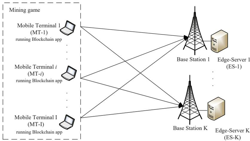
**Figure 1.** System model: a group of mobile terminals offload computational workloads to the edge servers.
