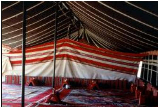
*Fig. 6. Interior of new tent in Haneedh, showing many departures from tradition. Metal poles replace wooden ones; the design of the roof is non-traditional for this area; the locally-made tent divider is hung from a high ceiling, whereas it would formerly have been hung from tent poles, with a low ceiling; cushions, arm rests and rugs are of foreign manufacture. 1993.*
