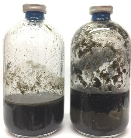
Figure 3. Municipal wastewater collected from the Theresa Street Water Resource Recovery Facility in Lincoln, Nebraska. (Left) Organic solids before anaerobic digestion. (Right) Organic solids after anaerobic digestion.
