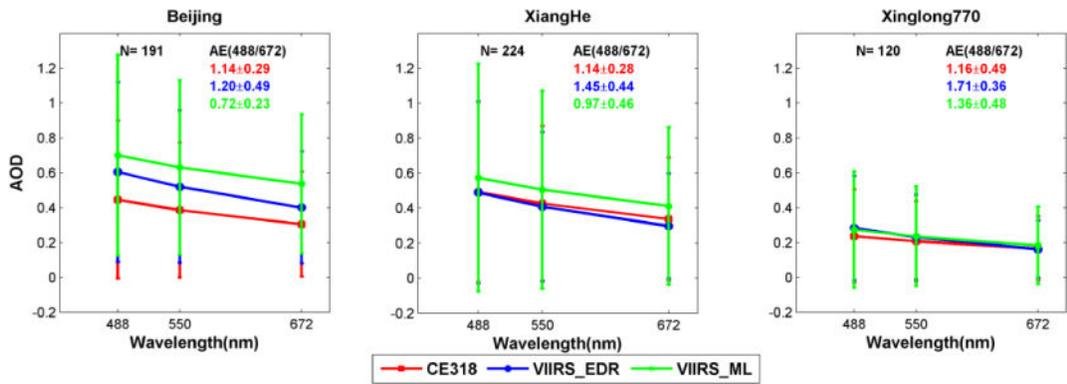
**Figure 1.** The average AODs of matchup data at blue (488 nm), red (672 nm) and 550 nm wavelengths between VIIRS\_EDR, CE318 and VIIRS\_ML. N is the number of matchup data. The average and standard deviation of Angstrom Exponent (AE) from 488nm and 672 nm of each matchup data set is also shown in this figure: red for CE318, blue for VIIRS\_EDR, and green for VIIRS\_ML.
