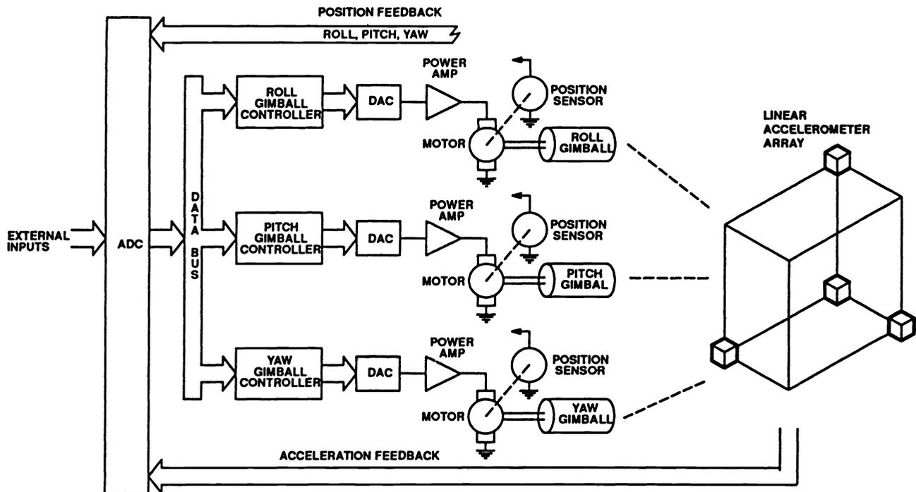
Fig. 4 Control system block diagram.
