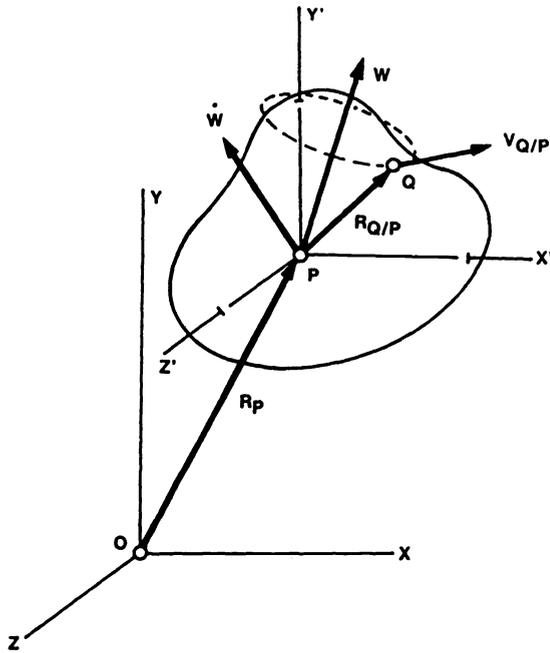
Fig. 1 Three-dimensional motion of rigid body.
