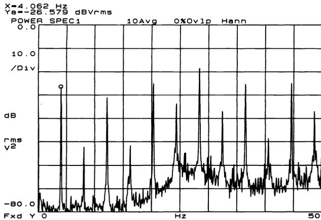
Fig. 9 Stabilized platform residual motion power spectrum.
