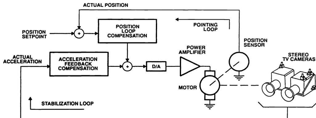
Fig. 5 Single-axis gimbal controller block diagram.
