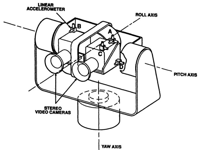
Fig. 3 Stabilized imaging sensor suite.
