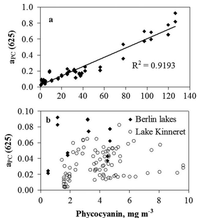
**Fig. 4.** Relationship between PC concentration and PC absorption at 625 nm in (a) Berlin lakes (all data), and (b) in Lake Kinneret and Berlin lakes as PC concentration in latter was below  $10 \text{ mg m}^{-3}$ . PC net absorption was calculated by Eq. 5.
