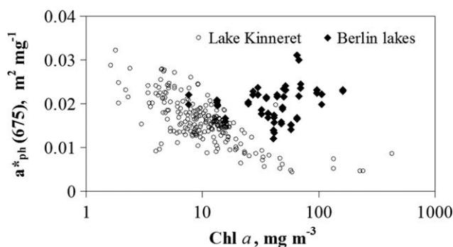
**Fig. 5.** The relationship between Chl *a* concentration and Chl *a* specific absorption coefficient at 675 nm,  $a_{\text{ph}}^*(675)$ , in Lake Kinneret and Berlin lakes. The relationship in Lake Kinneret was  $a^* = 0.342 \times [\text{Chl } a]^{-0.3463}$ , with  $r^2 = 0.564$ ,  $n = 348$ ,  $p < 0.001$ . Kinneret results include data collected in the current study and another 260 sample collected in previous years, to increase the range of Chl *a* concentration in the analysis.
