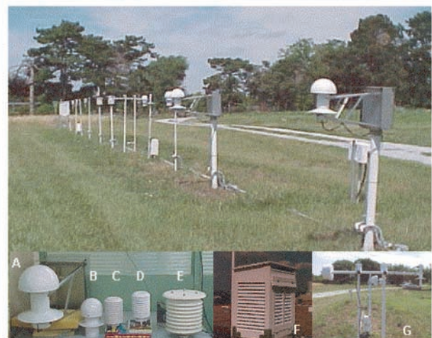
Figure 1. From upper right, the array of air temperature systems used (ASOS, ASP-ES, RMY, MMTS, Gill, NON-ES, and CRS shields) at the experimental field. The bottom shows all air temperature radiation shields individually with labels A, B, C, D, E, F, and G depicting the ASOS, ASP-ES, NON-ASP-ES, Gill, MMTS, CRS, and R. M. Young aspirated radiation shields.
