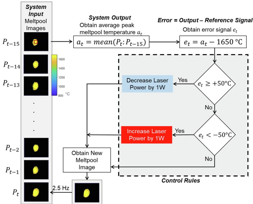
**Fig. 8.** Block diagram of the rule-based controller used to maintain the meltpool at a peak temperature of 1650 °C. The average of the peak meltpool temperature ( $a_t$ ) was taken over a trailing 16 readings. Then the error ( $e_t$ ) from 1650 °C was found and the laser power was adjusted accordingly. Then the new meltpool reading was recorded, repeating at a rate of 2.5 Hz.
