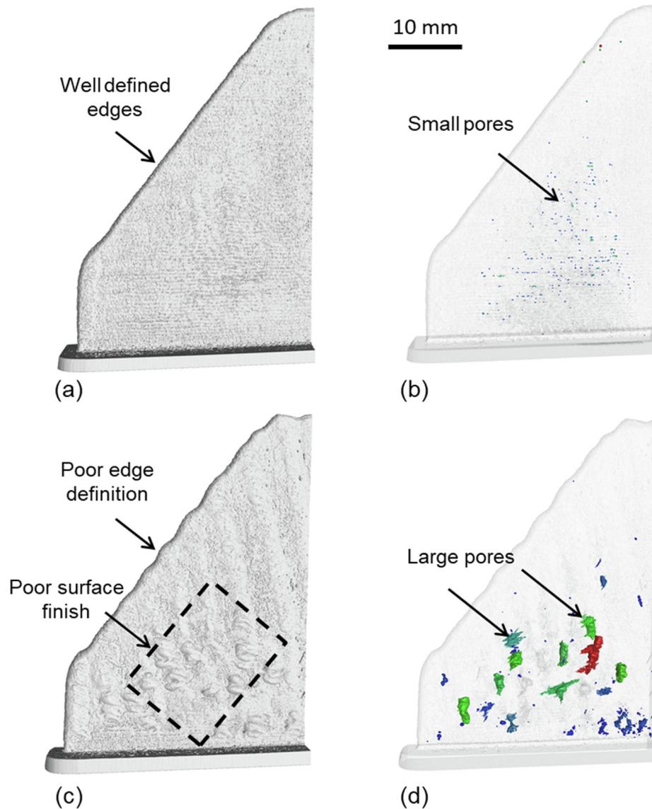
**Fig. 2.** An example of stochastic flaw formation in DED. X-ray CT scans of two stainless steel parts produced under identical DED processing conditions ( $P = 325$  W,  $V = 8.5$  mm·s<sup>-1</sup>). The part in (a) and (b) depicts near ideal surface finish and few, small pores. The part in (c) and (d) shows poor surface finish, degraded geometry, and large pores.
