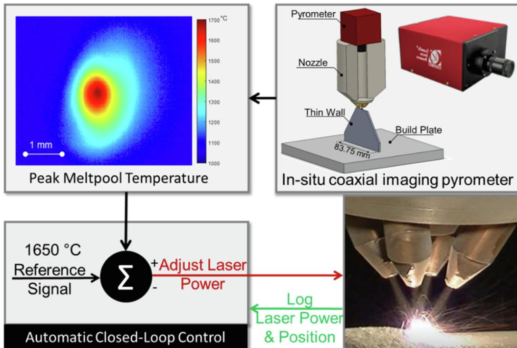
**Fig. 7.** Control-Loop used to maintain the peak melt pool temperature at 1650 ± 50 °C using a Stratronics two-wavelength imaging pyrometer and Optomec's Lens MR7 DED machine. The peak melt pool temperature is measured in a 10 pixel × 10 pixel square surrounding the center of the melt pool image. The laser power is adjusted proportional to the peak melt pool temperature. The system logs the position of the nozzle and the adjusted laser power.
