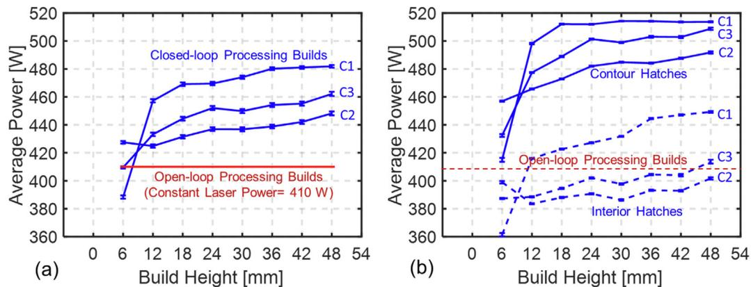
**Fig. 15.** (a) Trend of laser power in closed-loop processing relative to open-loop processing (b) difference in the laser power between contour and interior hatches of closed-loop processing with respect to open-loop processing. Error bars show the mean  $\pm$  1 standard error.
