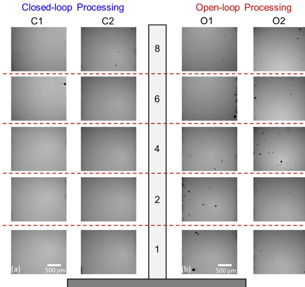
**Fig. 16.** The optical micrography images for two closed-loop processed parts (C1 and C2) and open-loop processed parts (O1 and O2) across the 8 sub-sections. (a) The pores observed in closed-loop processed parts are consistent in size and occurrence. (b) In open-loop processed parts the number and size of the pores varies both within and between parts.
