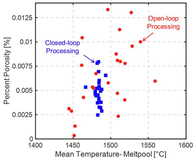
**Fig. 20.** Scatter plot comparing the mean temperature of the meltpool region to the percent porosity in all sub-sections of Sample A and B. Both closed-loop and open-loop processed parts are plotted to give a full comparison. All three closed-loop processed parts stay clustered due to the constancy between and within parts. open-loop processed parts are scattered due to minimal constancy between parts.
