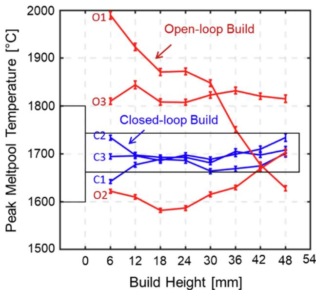
**Fig. 11.** Comparison of the peak meltpool temperature for the open-loop and closed-loop processed parts. The peak meltpool temperature for the parts processed under open-loop conditions (fixed laser power of 410 W) varies from ~1560 to 2000 °C. In contrast, the peak meltpool temperature for the parts built with closed-loop control of the laser power remains within 1650 ± 50 °C. Error bars show the mean ± 1 standard error.
