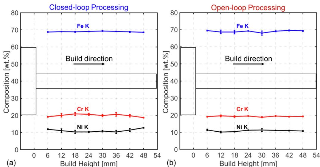
Fig. 28. EDS point analysis of as-built SS 316L parts. There is no discernable change in the elemental composition (wt.%) within and between parts deposited using either (a) Closed-loop processing, and (b) open-loop processing as a function of build height. Error bars show the mean  $\pm$  1 standard error.
