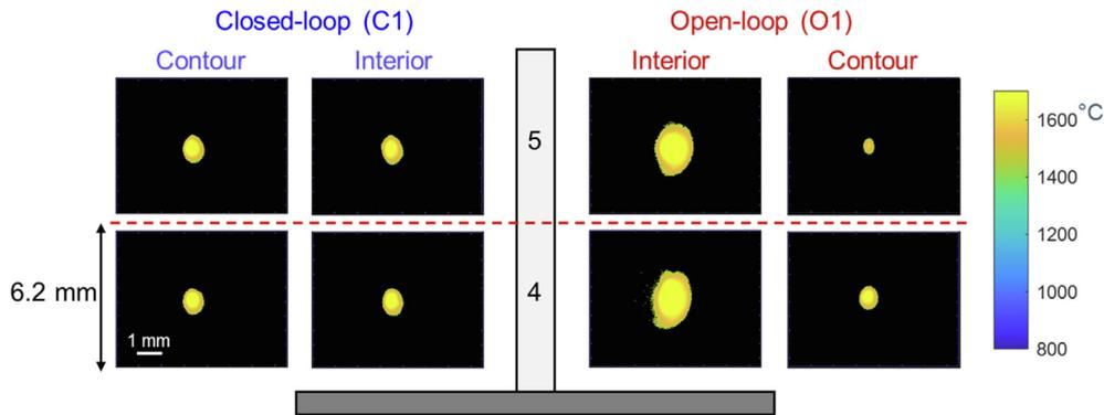
**Fig. 14.** Visual representation of the shape of the meltpool region at the two central sub-sections of the build, for the closed-loop and open-loop processed parts C1 and O1, respectively. The meltpool shape varies considerably for the open-loop processed part O1. Each pyrometer image is randomly selected for each sub-section.
