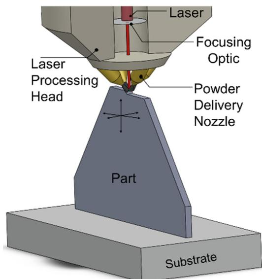
**Fig. 1.** Schematic of the P-DED process. Material in the form of metal powder is sprayed from the sides by four nozzles and fused onto a substrate by energy from a coaxial laser beam.
