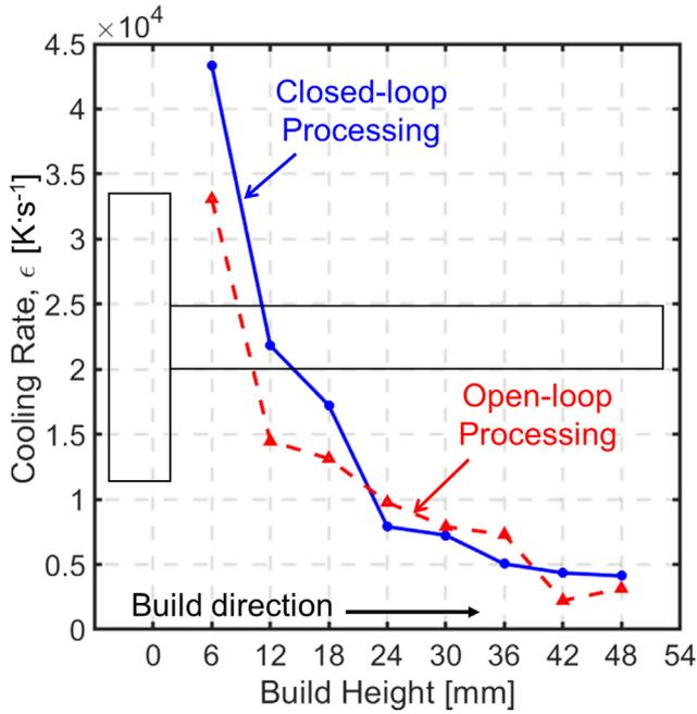
Fig. 24. The mean cooling rate,  $\epsilon$ , measured from the primary dendrite arm spacing at 8 different sections along the build. The data is representative of parts O1 and C1.
