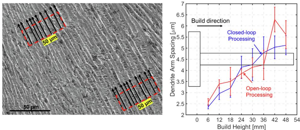
**Fig. 23.** (a) Measurements of primary dendrite arm spacing (PDAS) for a representative SS 316L build C1. A representative SEM image of the dendritic microstructure from which PDAS were measured; (b) Primary dendrite arm spacings as a function of build height for representative parts O1 and C1. Error bars show the mean ± 1 standard error.
