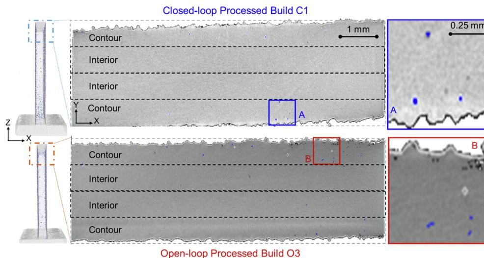
**Fig. 19.** Visual comparison of porosity from representative XCT slices between build C1 (A) and O3 (B). Notice that there are more pores on the contour hatches relative to the interior hatches for both closed-loop and open-loop processed parts.
