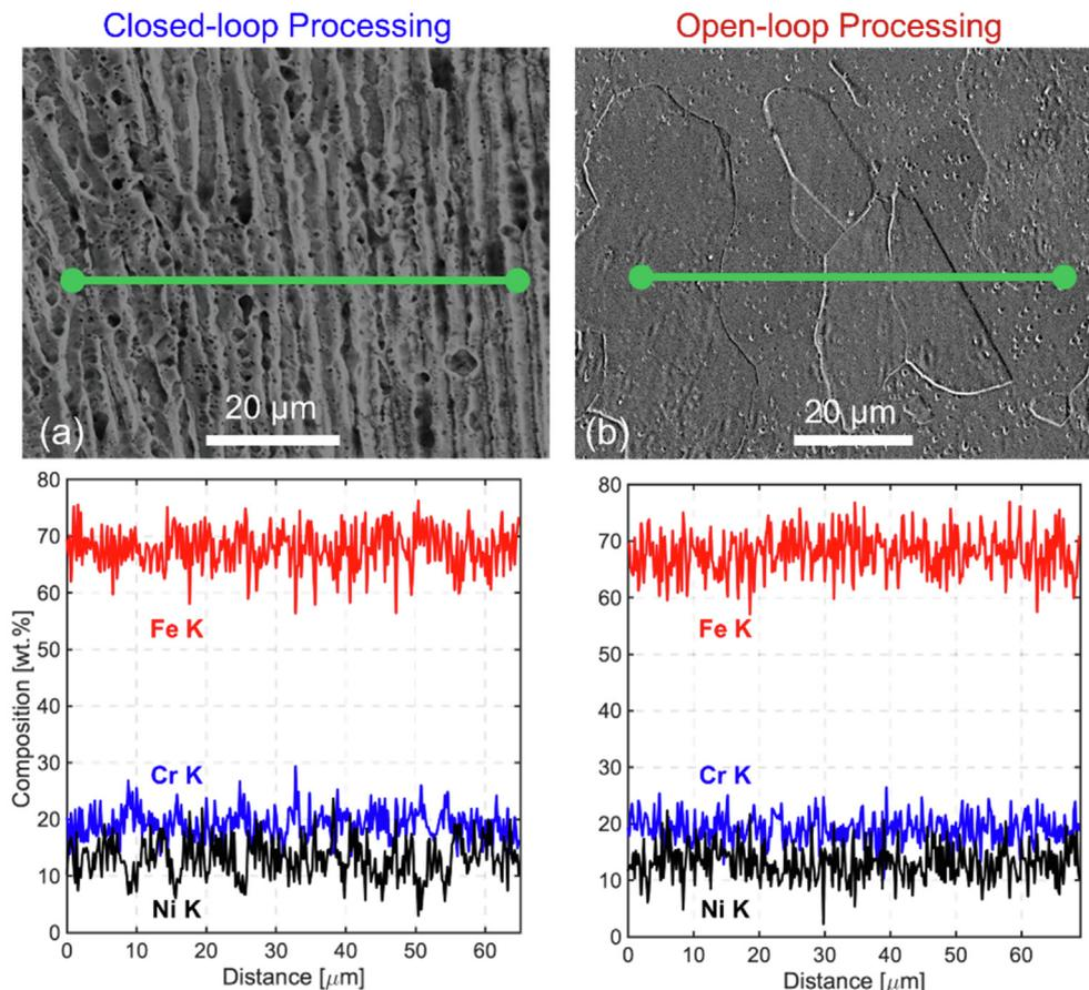
**Fig. 29.** EDS line scan analysis of different microstructures from (a) Closed-loop processing and (b) open-loop processing. The elemental composition is uniform within the parts and there is no variation in elemental composition between the two processing methods, albeit the microstructure evolved is different. EDS data were collected from samples O1 and C3.
