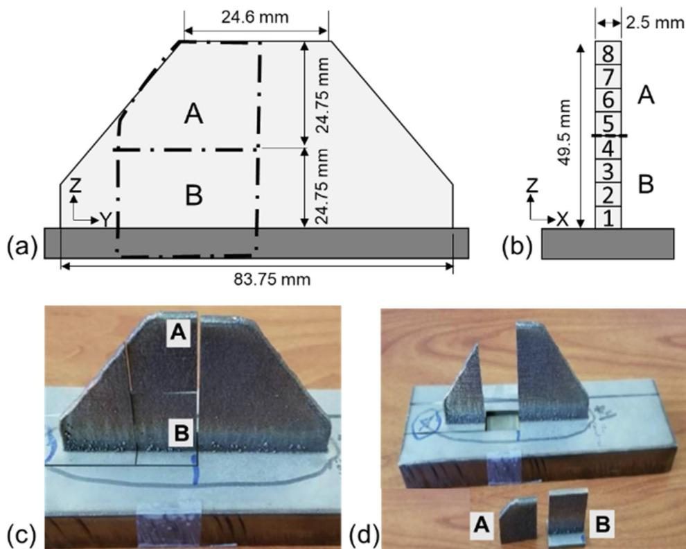
**Fig. 9.** (a and b) Schematic and (c and d) pictures of the part cut into sample A and sample B in order to perform metallurgical analysis. Sample A is the top cross-section and Sample B is the bottom cross-section. The part is divided into 8 sub-sections of 6.2 mm height for analysis.
