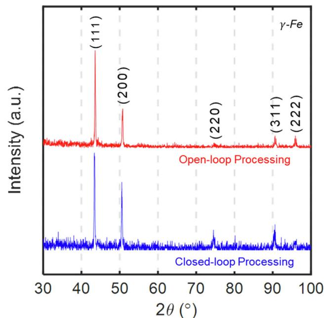
**Fig. 27.** X-ray Diffraction patterns of as-built SS 316L parts using closed-loop (blue) and open-loop (red) processing methods. The two types of parts have a single phase ( $\gamma$ -Fe). There is no difference in the microstructure phases between closed-loop and open-loop processing. (For interpretation of the references to color in this figure legend, the reader is referred to the web version of this article.)
