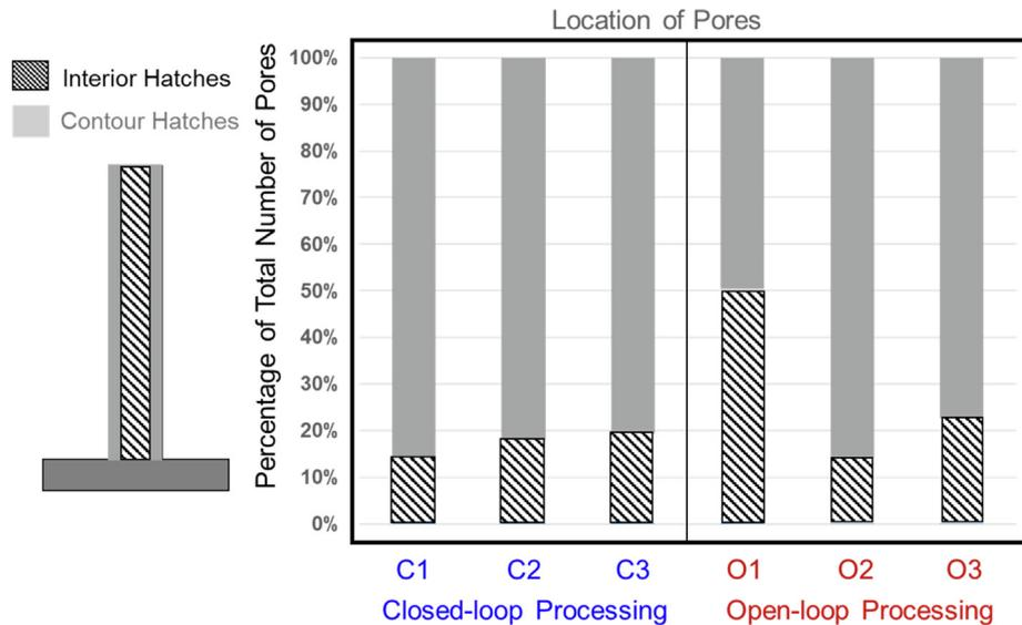
**Fig. 18.** Stacked bar charts comparing the location of pores between the contour (gray) and interior (black & white striped) hatches. Then comparing the distribution of pores between closed-loop processed parts (left) and open-loop processed parts (right).
