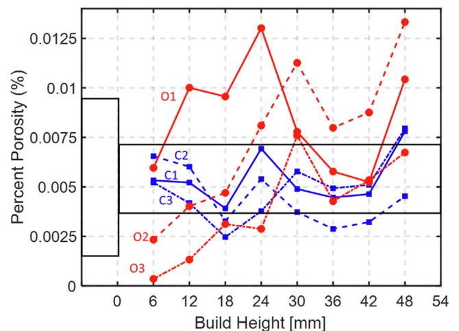
**Fig. 17.** The volume percent porosity obtained using non-destructive X-ray computed tomography (XCT) analysis for the closed-loop and open-loop processed parts tracked as a function of the build height. The closed-loop processed parts have a consistent percentage porosity throughout the build height compared to the large variation observed in open-loop processed parts.
