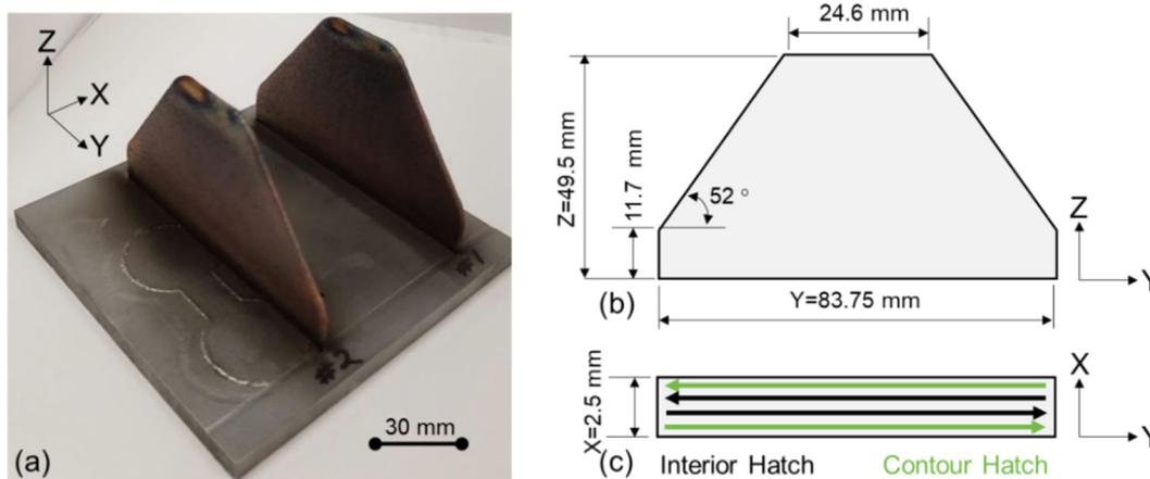
**Fig. 3.** (a) Photograph of as built SS 316L parts used in this work and (b) The dimensions of the trapezoidal parts. (c) The deposition and scan pattern under which the parts are produced. The substrate is stainless steel and 12.7 mm thick. The parts shown in this figure were produced under open-loop processing conditions; burn marks are noted near the top of these parts as a consequence of overheating.
