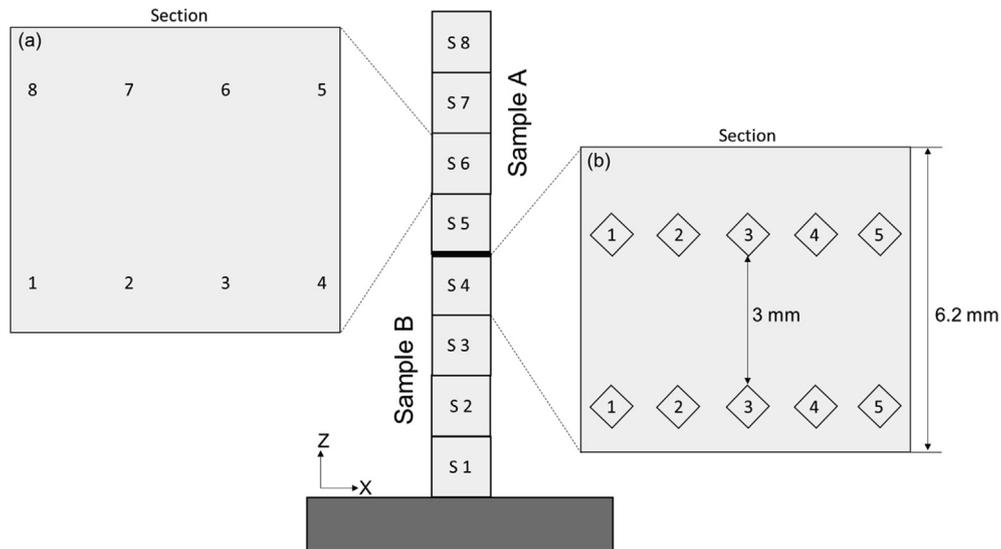
**Fig. 10.** Schematic of a part divided into eight sub-sections, labeled S1 through S8. Each sub-section is 6.2 mm tall and 2.5 mm wide. Schematic of locations (a) where the SEM images were taken to perform grain morphology analysis and (b) where microhardness readings were taken for each sub-section.
