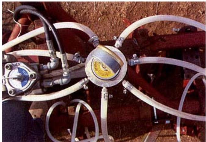
**Figure 6. Anhydrous ammonia distribution manifold with outlets equally spaced around the manifold.**
