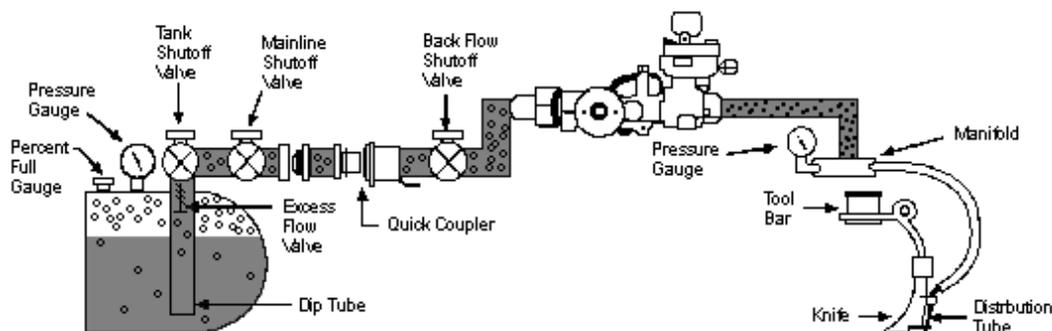
**Figure 4.** Schematic drawing of components for a typical anhydrous ammonia applicator.
