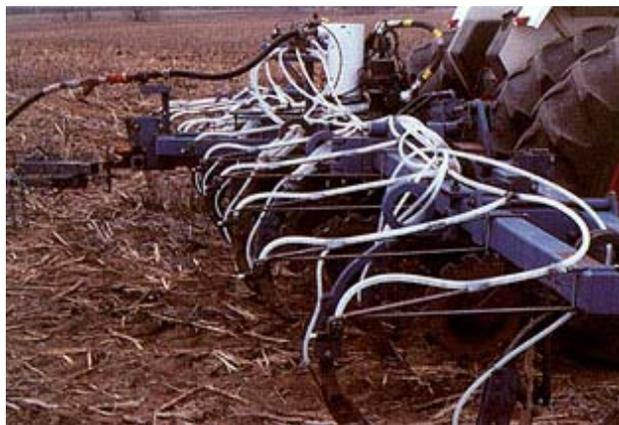
Figure 8b. Anhydrous ammonia applicator equipped with vibrating shank knives.
