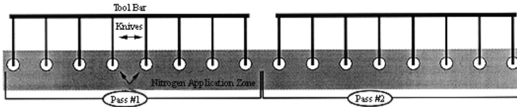
**Figure 9a.** Two passes of an 8-knife applicator without overlap of outside knives suitable for preplant applications.
