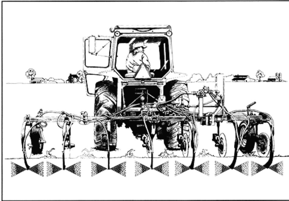
**Figure 7a.** Conceptual drawing of uniform application due to manifold being level.
