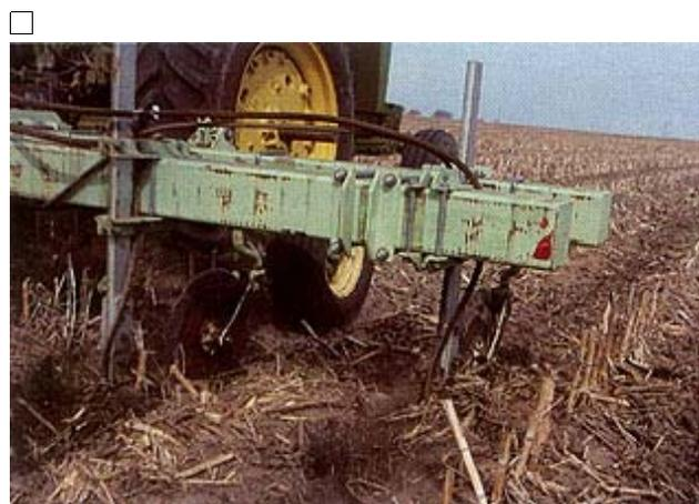
**Figure 8a. Anhydrous ammonia applicator equipped with straight shank knives.**
