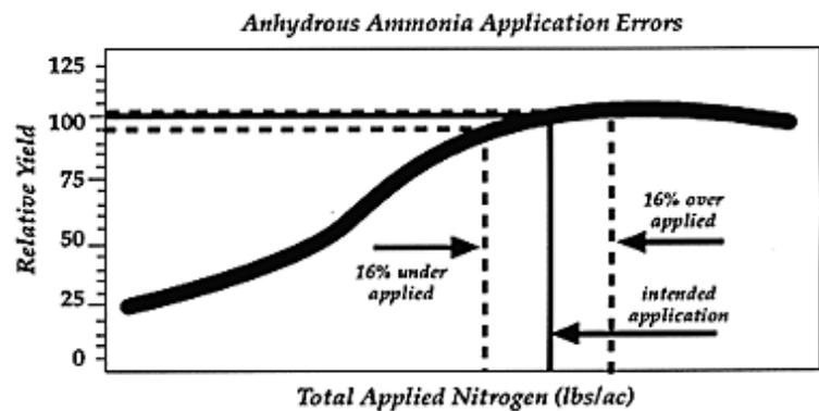
Figure 1a. Potential variation in anhydrous ammonia application rates using regular type application equipment.
