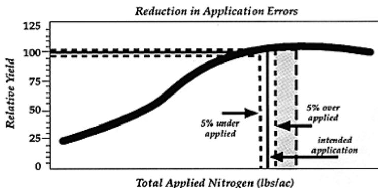
Figure 1c. Potential reduction in anhydrous application rate due to knowledge that variation in the field application rate is 5 percent or less. The shaded portion represents the anhydrous savings due to reduced variation in application rate compared to 16% error.
