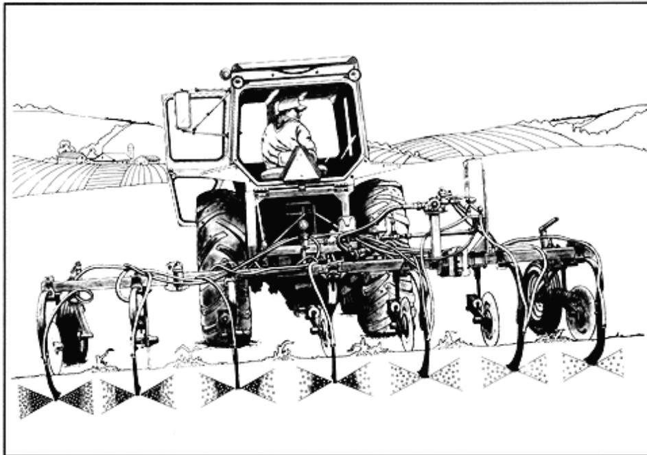
**Figure 7b.** Conceptual drawing of the variation in applicator knife output due to manifold being tilted.
