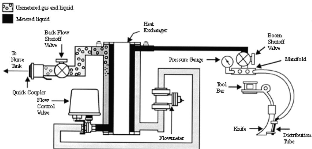
**Figure 5b. Components of a flow control monitor metering device including the tank, thermal transfer unit, control valve, and flow meter. (Adapted from drawing by Dickey John Corporation)**
