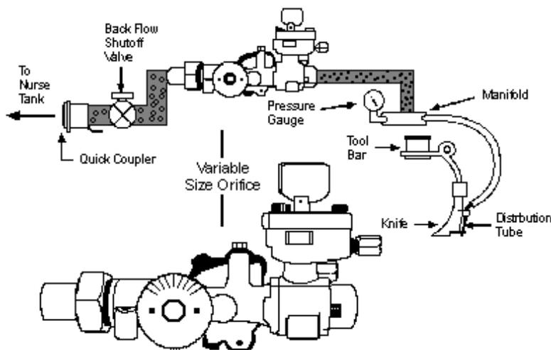
**Figure 5a. Components of a variable size orifice metering device including the tank discharge, regulator, manifold, and knife applicator. (Adapted from Continental  $\text{NH}_3$  Products Company, Inc.)**
