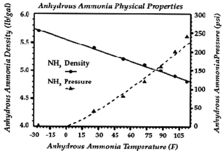
Figure 3. Change in anhydrous ammonia density and pressure with increasing temperature.
