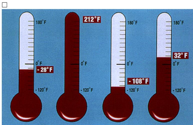
Figure 2. Temperatures at which anhydrous ammonia and water will boil or freeze.
