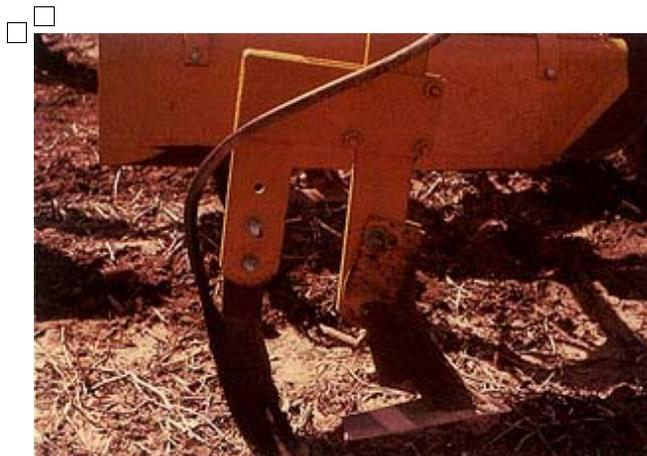
Figure 8c. Anhydrous ammonia applicator equipped with behind cultivator sweep knives.
