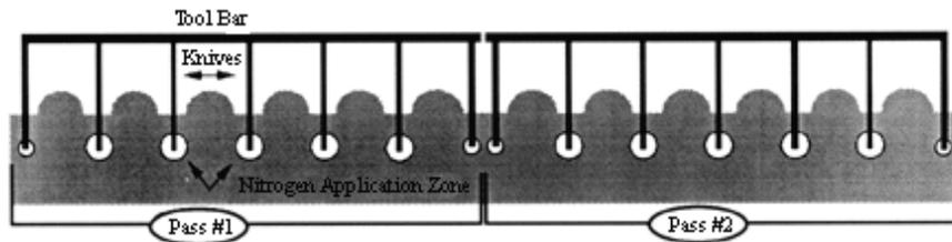
**Figure 9b.** Two passes of a 7-knife applicator in a field planted with a six-row planter showing overlap of two outside rows.
