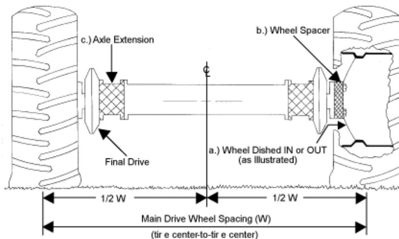
Figure 3. Wheel spacing adjustment for combine drive axle. Also available are: a) wheel dish "in" and "out", b) wheel or hub spacers, c) axle extensions for the final drives.
