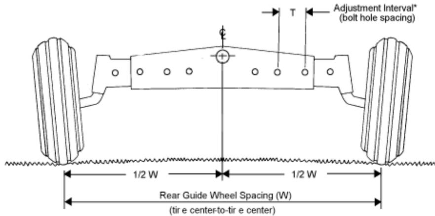
Figure 2. Adjustable rear steer axle for self-propelled combines. Some fixed axles allow wheels to dish "in" or "out" for two possible wheel spacings.
