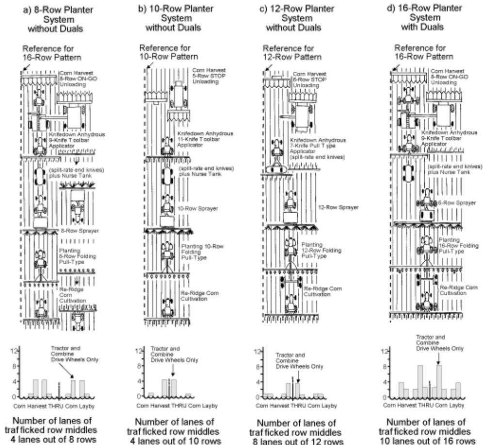
Figure 6. Traffic patterns using 8-, 10-, 12-, and 16-row equipment systems. None of these equipment systems were equipped with duals. From left to right: a) 8-row equipment system with all 8-row equipment and on-the-go unloading, b) 10-row equipment system using an odd-row header and spacing width is the same for combine and tractors, no on-the-go unloading, c) 12-row equipment system, no on-the-go unloading, d) 16-row equipment system with on-the-go unloading.
