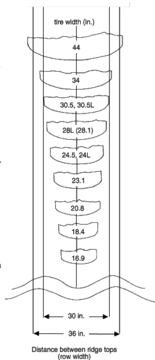
Figure 4. Combine tire size within ridge profiles. Minimize ridge deformation with proper tire sizing and spacing.
