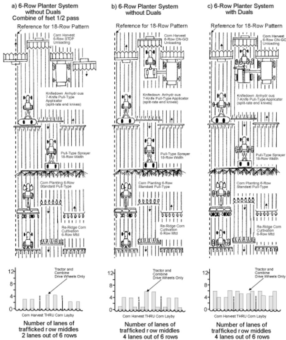
Figure 5. Traffic patterns using 6-row equipment systems. From left to right, a) center combine on guess row, no grain fill vehicles in the field, b) equipment system that uses singles with on-the-go unloading, c) equipment system that uses duals and on-the-go unloading.
