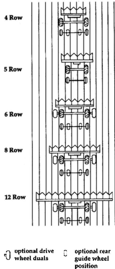
Figure 1. Combine row crop header size and wheel spacing combinations. The outer edge of the drive wheels on the 4- and 6- row (using straddle duals) may extend past the header and could run very close to the next unharvested row. May require tire shielding and superior driving skills.
