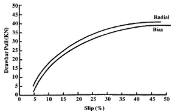
**Figure 3. Drawbar curves for radial and bias-ply tire (18.4-38 R-1 Size) operating in untilled soil.**
