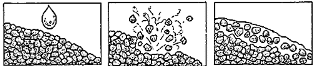
Figure 2. Soil particles and aggregates that have been detached by raindrops are transported down the slope by runoff.
