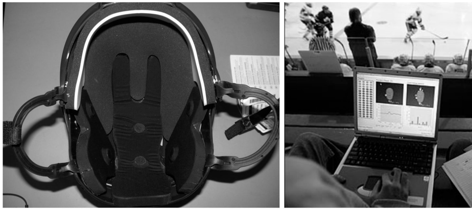
Figure 1. The Head Impact Telemetry (HIT) System was used to record frequency, location, and severity of head impacts in ice hockey. Left: Inside view of an Easton S9 equipped with an instrumented helmet unit (IHU). Right: A rink-side antennae connected to a laptop computer actively communicates with IHU to collect and process impact data received via radio transmitter.
