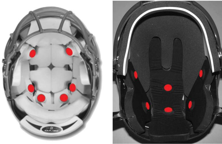
Accelerometer locations (indicated by red circles) within the instrumented football and hockey helmets record acceleration at 6 locations on the head. Raw acceleration data for each recorded event are processed using an optimization algorithm to obtain linear and rotational acceleration about the head center of gravity.
