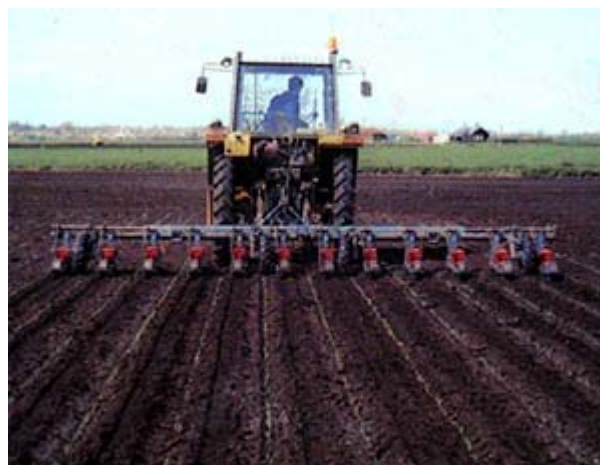
Figure 4. Sugarbeets are being planted into a spring seeded cover crop that was planted with the same planter.
