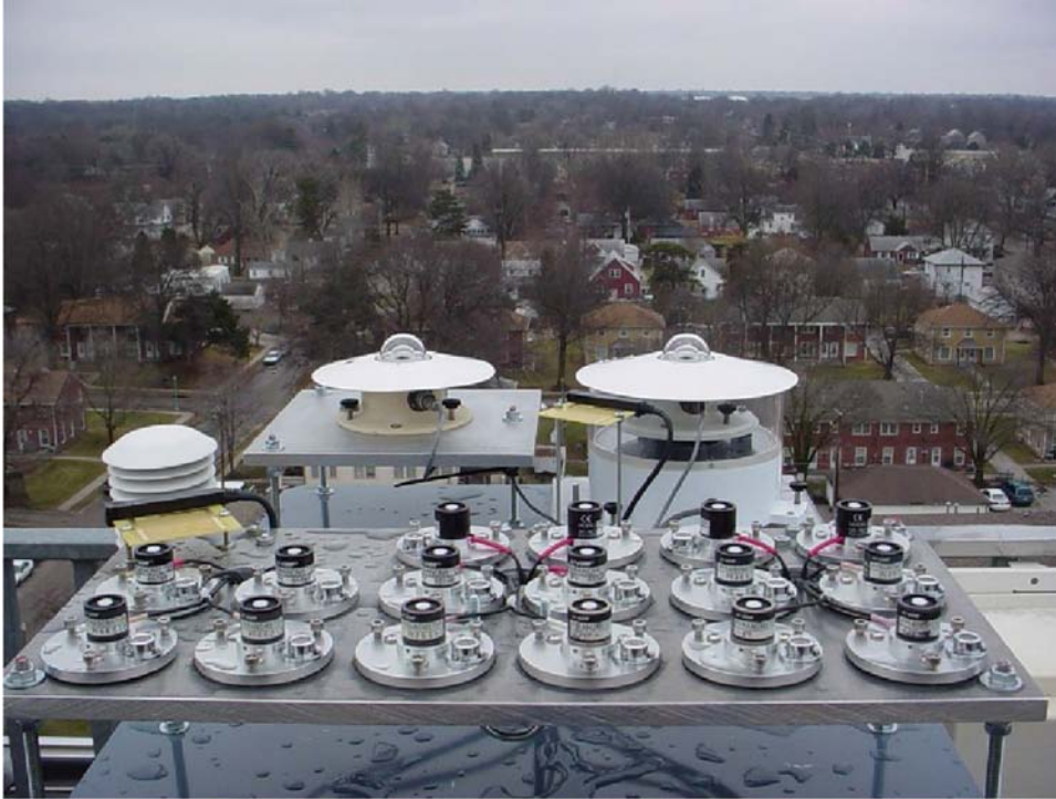
Fig. 1. Pyranometers mounted on the aluminum plate surface of a leveling table on the roof of a nine-story building (Hardin Hall, University of Nebraska-Lincoln). The silicon photodiode pyranometers are in the foreground and the Eppley precision spectral pyranometers (PSPs) are in the background. An air temperature thermistor and its shield are in the back left.
