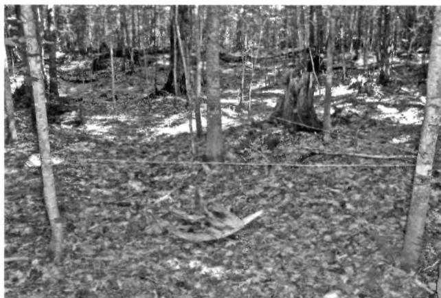
FIGURE 1. Snare configurations used to obtain hair samples from free-ranging white-tailed deer. Top panel is a 60 x 60 cm barbed wire hair snare positioned 46 cm above ground. Bottom panel is a barbed wire snare stapled to three trees 80 cm above ground level.
