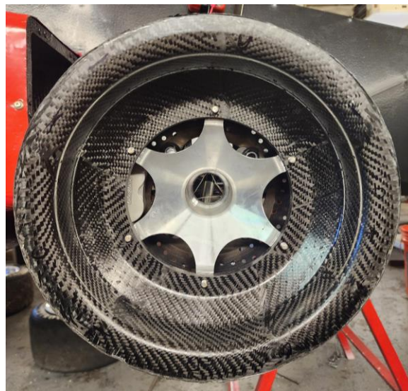
Figure 1. Finished carbon one-piece wheel mounted to the 2024 competition car.
