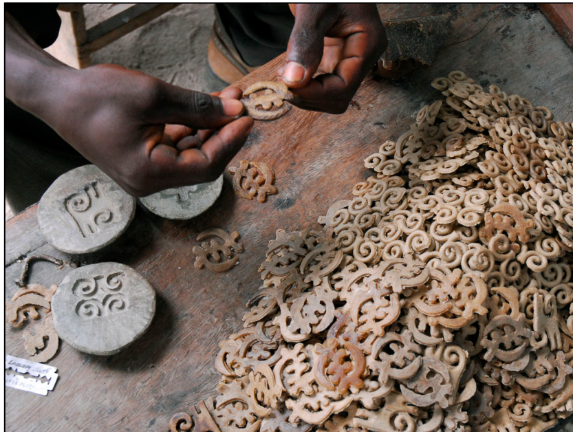
Figure 2. Ashanti wax models of Except God 7 (held in hands), Rams Horns 8 , and Bravery 9 being prepared for lost wax casting 10 in Krofofrom. Photo by Carol Ventura, Ghana, 2009.
