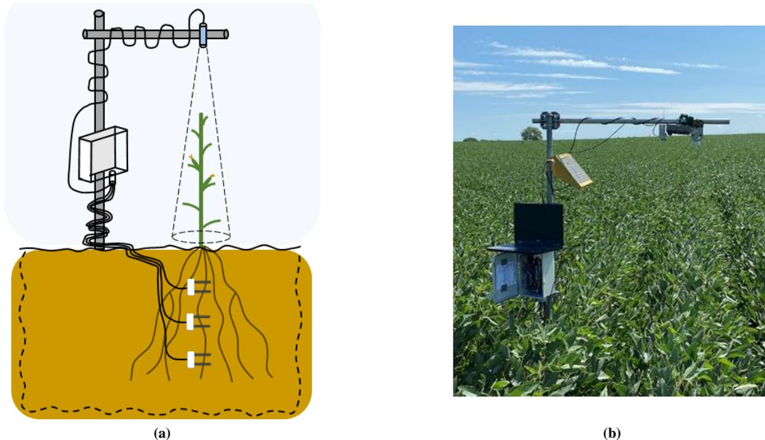
**Figure 1. (a) Illustration of sensor node station comprised of soil water sensors at 0.15 m, 0.46 m, and 0.76 m below the crop row and an infrared radiometer sensing the crop canopy maintained 1 m over the top of the maize canopy; (b) Sensor node station comprising of infrared radiometer sensor sensing the soybean canopy from 2 m above the ground.**
