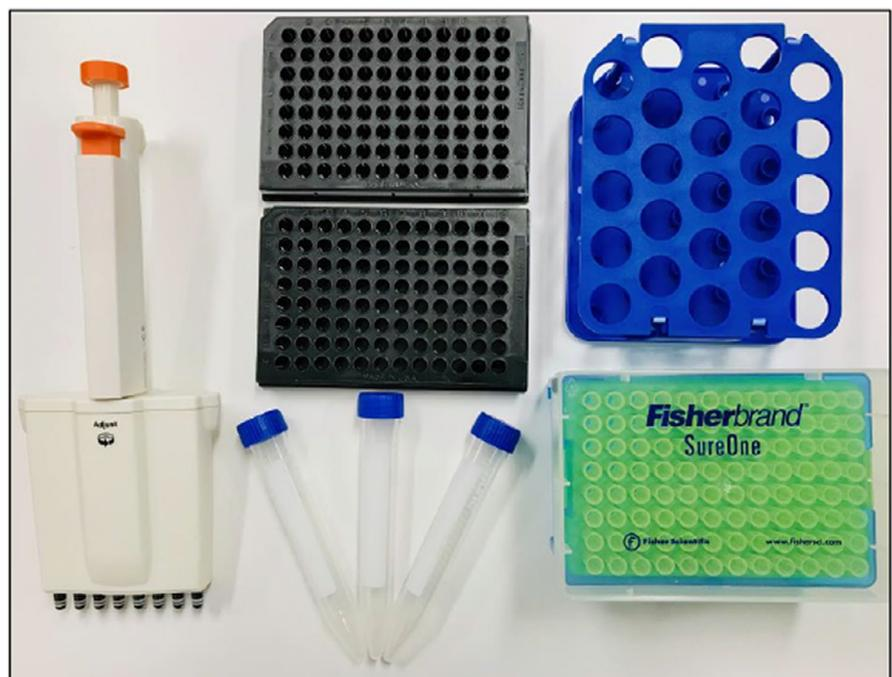
**FIGURE 2** Hardware needed for the high-throughput method detailed here: multi-channel pipette with autoclaved pipette tips, black 96-well plates, 15 ml centrifuge tubes with caps and holder.
