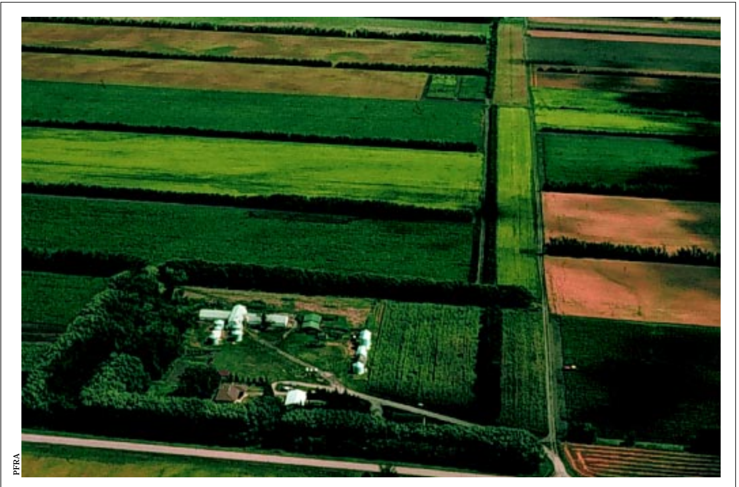
A well-designed farm or ranch incorporates many types of windbreaks to protect fields, livestock, and the homesite.
