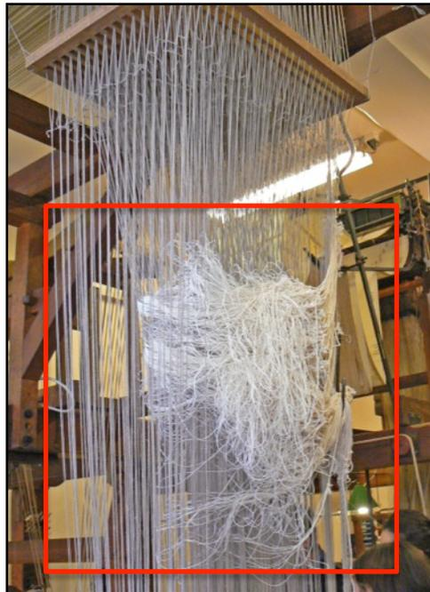
*Figure 1. Lashes tied on a drawloom simple at the Maison des Canuts, Lyon. This device permits successive groups of warp ends to be selected to form a pattern.*
