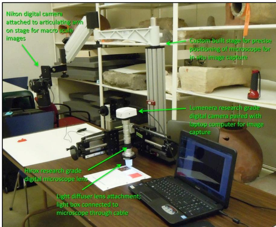
**Figure 3. Portable equipment setup for conservation-safe, cross-collection photographic documentation of weft-faced compound weave figured silks**
